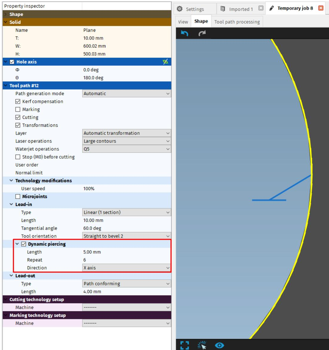
**Fig. 154: Lead-in with enabled dynamic piercing**
