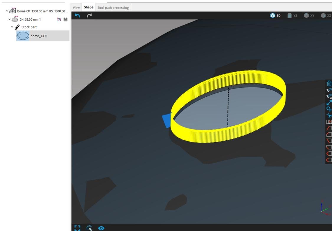
**Fig. 170: Reversed cut path with lead-in on the outer contour**
