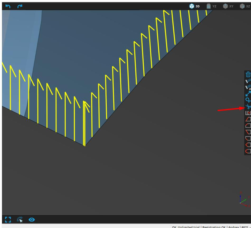
**Fig. 173: Splitting path using scissors in cut path editing widget**
