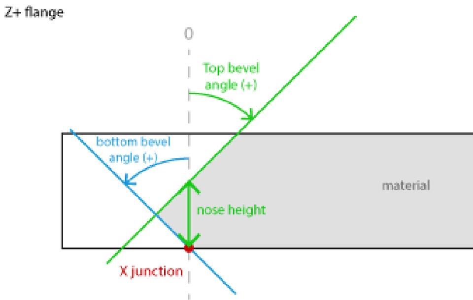
**Fig. 123: Z+ flange with bevel parameters**
