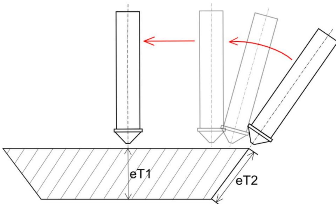
**Fig. 239: Effective cutting thickness**
