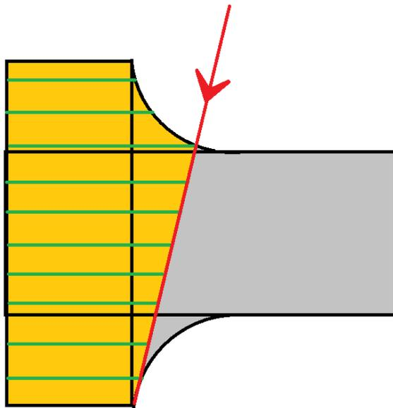
**Fig. 243: H – beam middle section cutting**
