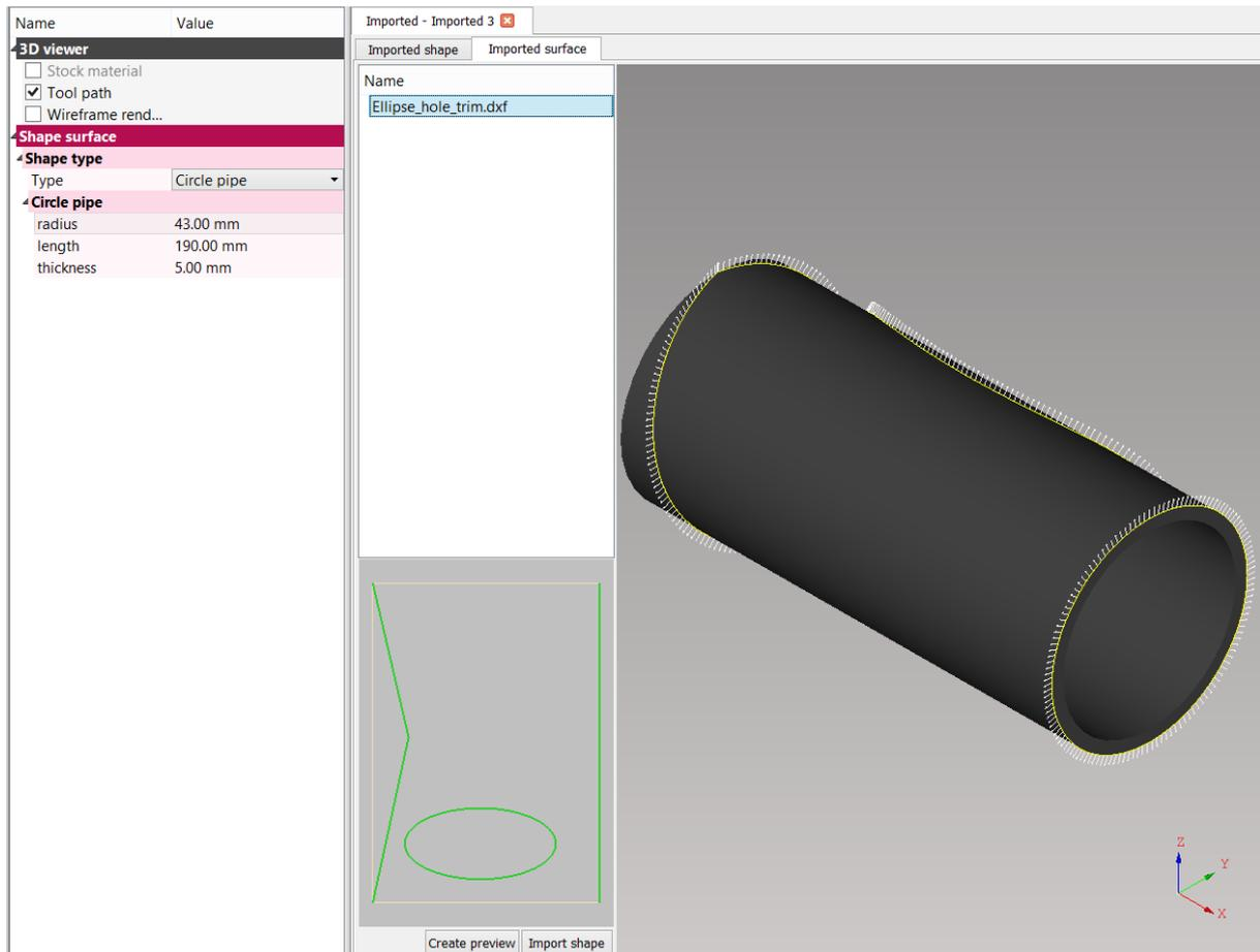
**Fig. 49: Importing of wrapped 2D surface around circle pipe**
