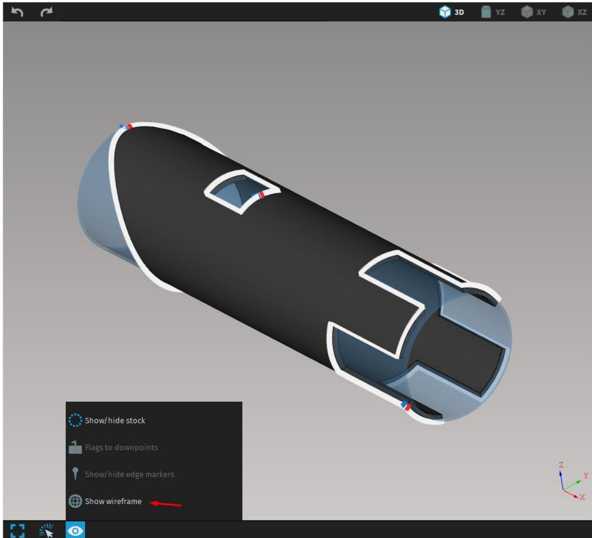
**Fig. 40: The option to display the part in wireframe rendering is located in viewer menu under the eye icon**
