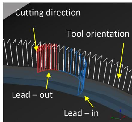
**Fig. 138: Cutting path and its sections**
