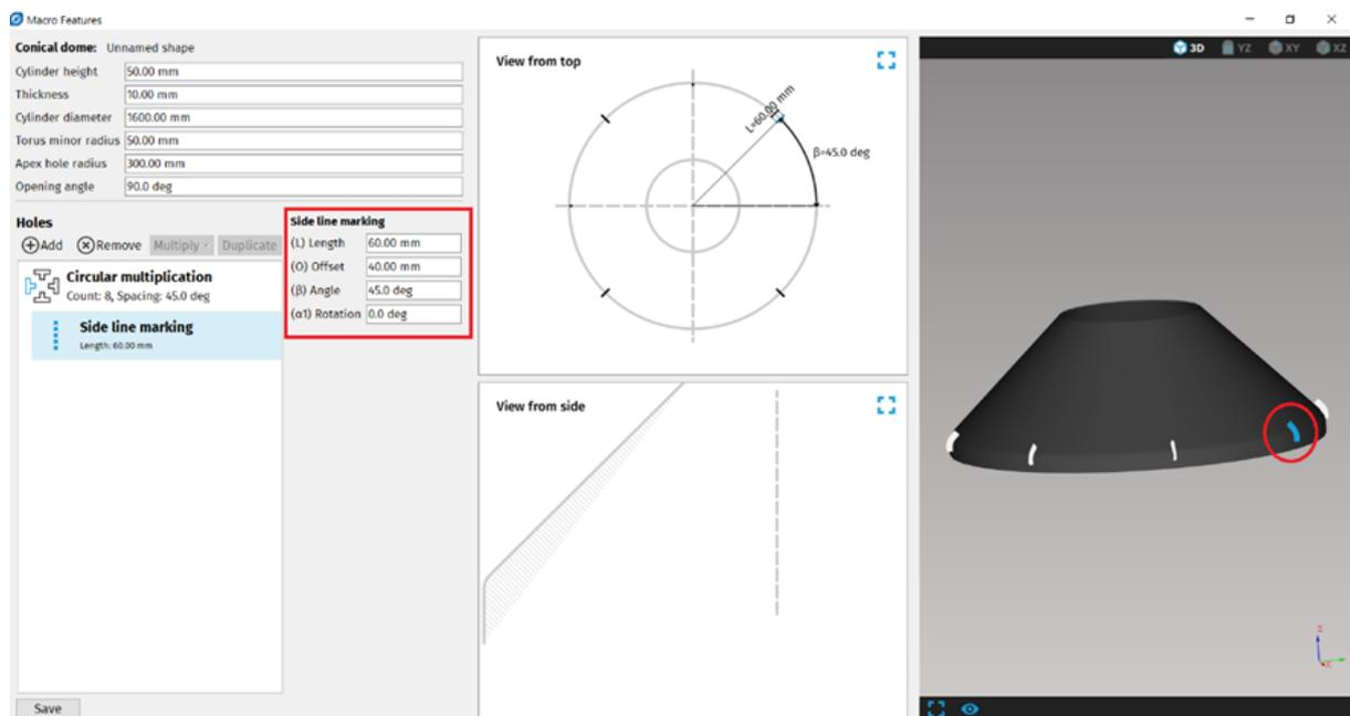
**Fig. 112: Example of Side line marking macro placed on Conical dome**
