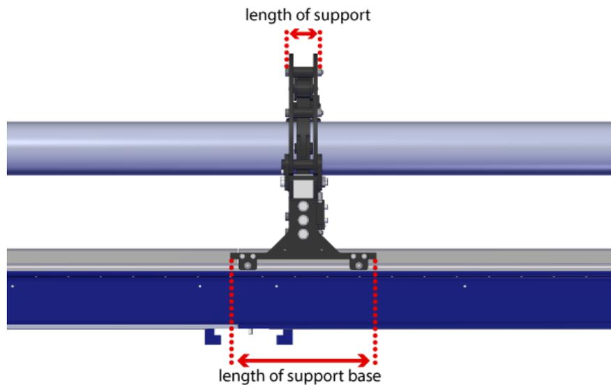
**Fig. 315: Length of support and support base**
