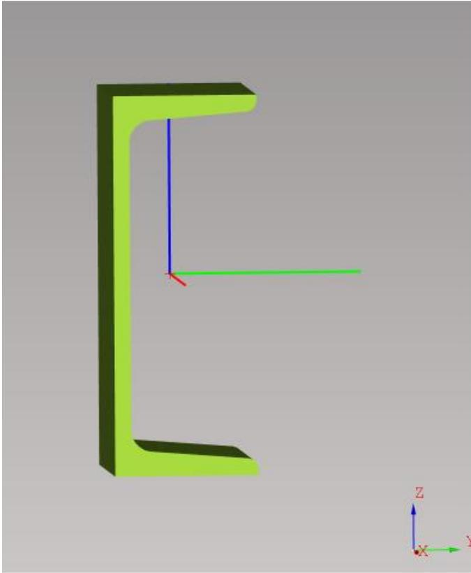
**Fig. 78: UPN bar (old position) Flanges are in Y axis with web facing in Y- direction**
