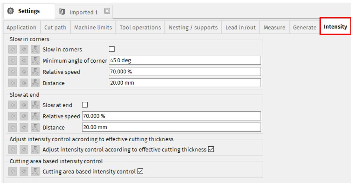
**Fig. 341: Intensity settings – cutting intensity modifiers**
