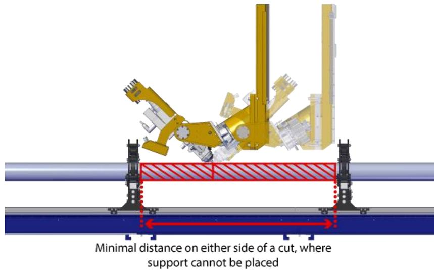
**Fig. 314: Blocked areas for cutting X+ and X-**
