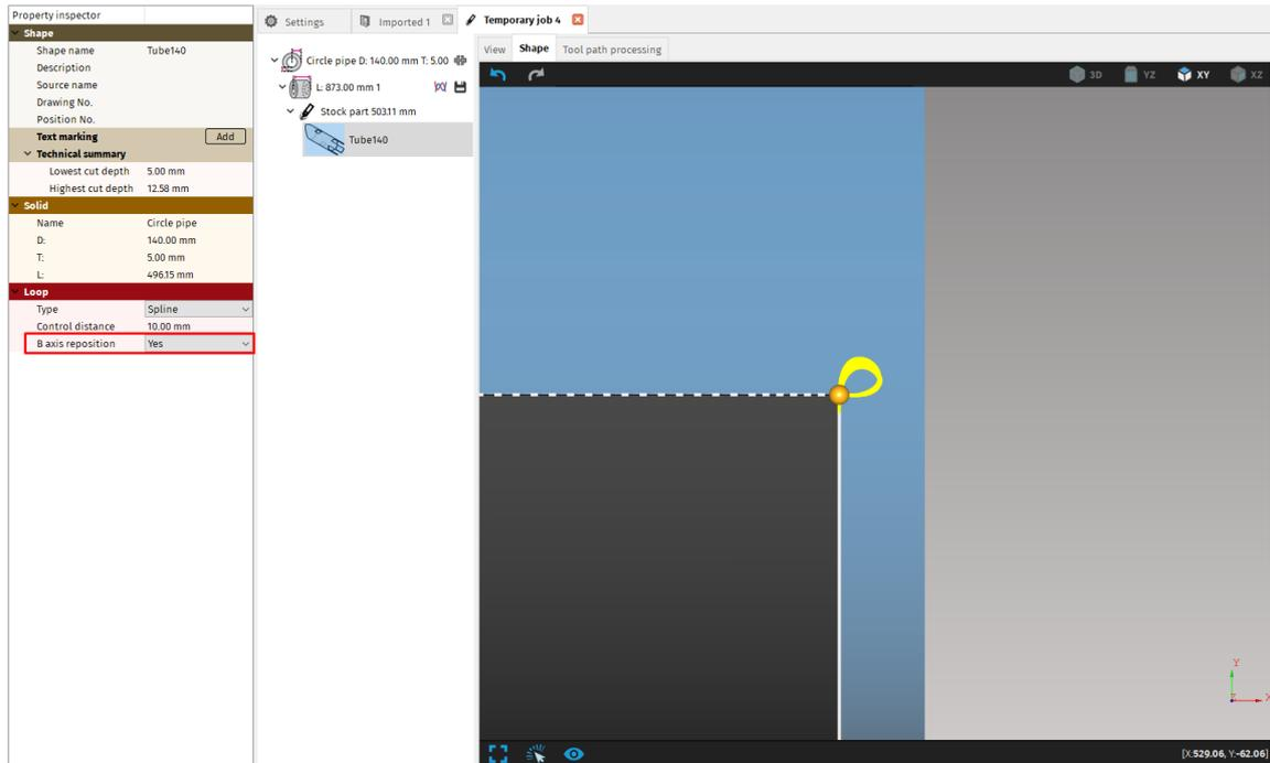
**Fig. 235: Example of loop wit B axis reposition enabled**
