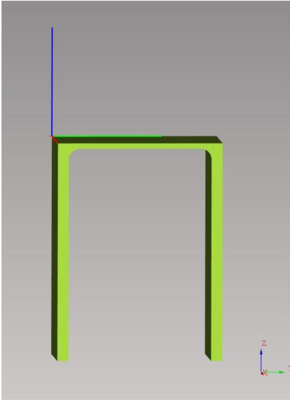
**Fig. 84: U-bar – Flanges are in Z-axis, with web facing Z+ direction**
