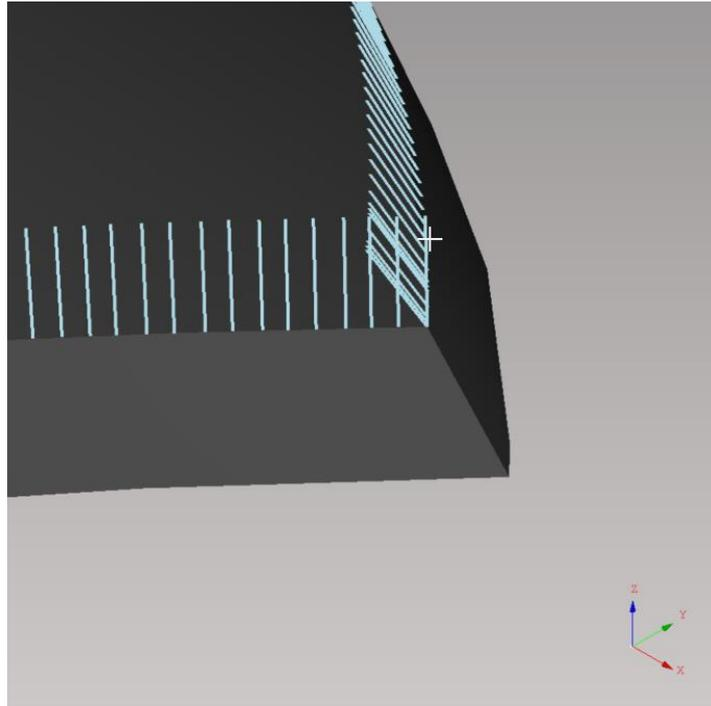
**Fig. 168: Selection of cutting path points to be erased**
