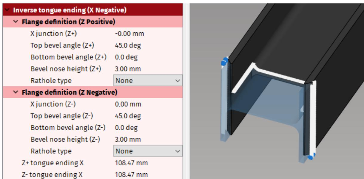
**Fig. 128: Inverse tongue ending and its parameters in Properties area**
