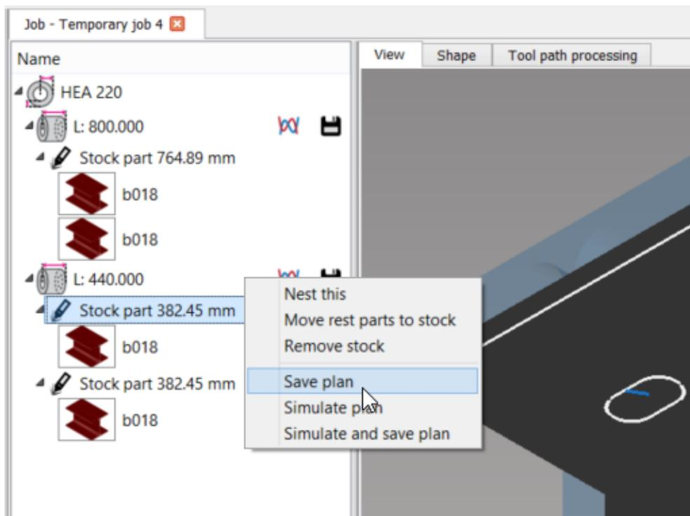
**Fig. 278: Save cutting plan for first stock part in stock with 440 mm**
