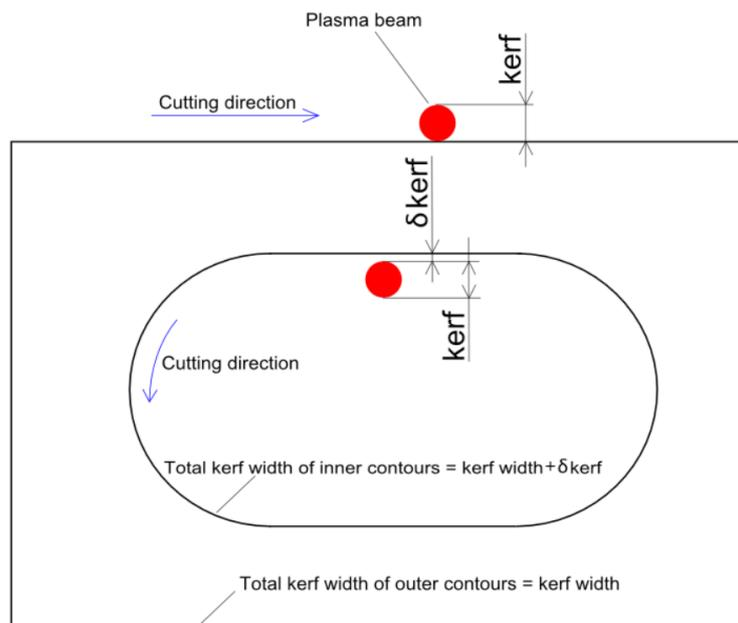
**Fig. 301: Delta kerf width for inner contours**
