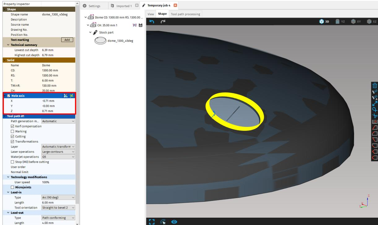
**Fig. 149: Hole axis properties**
