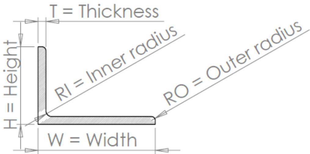
**Fig. 17: L beams (equal / unequal leg angles)**
