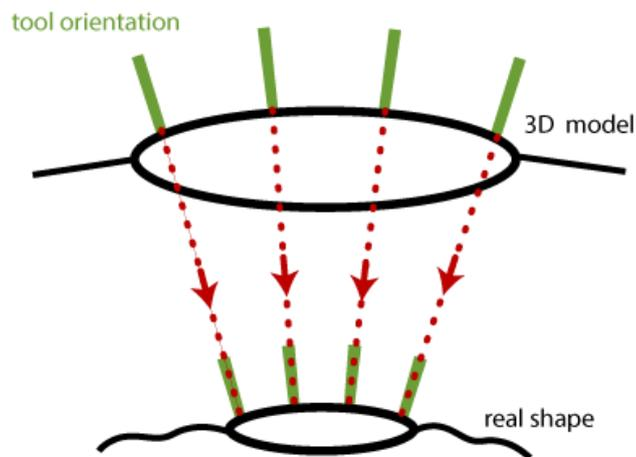
**Fig. 148: Direction of shifting the cutting path without generated hole axis**
