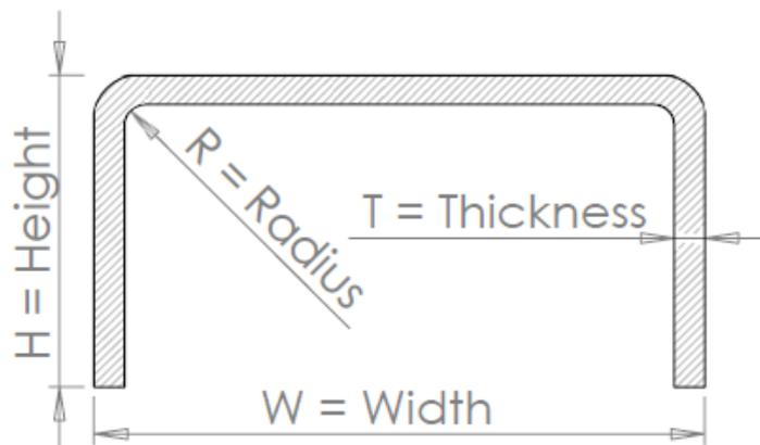
**Fig. 16: Bent U-beam**
