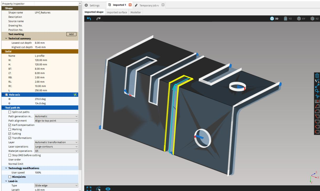
**Fig. 143: Align to top point – hole will maintain the distance from the edge that it is passing through**
