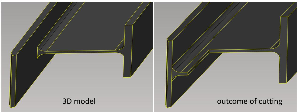
**Fig. 134: Difference between the 3D model and the real outcome of cutting**
