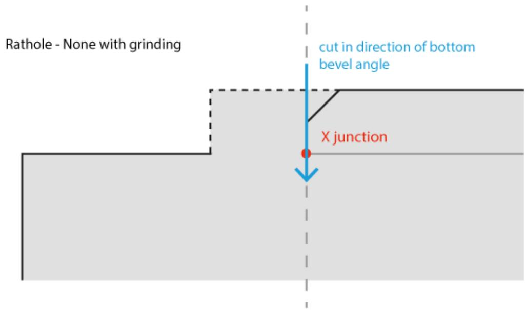
**Fig. 126: Rathole - None with grinding**
