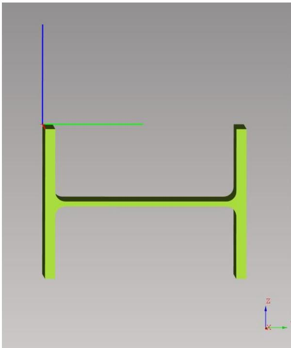
**Fig. 83: H-bar – Flanges are in Z-axis direction**
