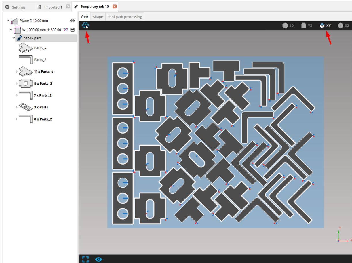
**Fig. 263: Manual nesting is activated and the view is locked in 2D top view**
