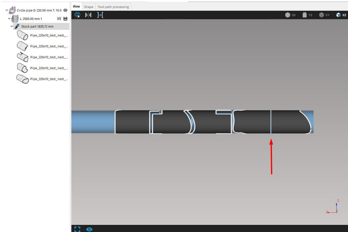
**Fig. 266: Parts nested with applied common cut**
