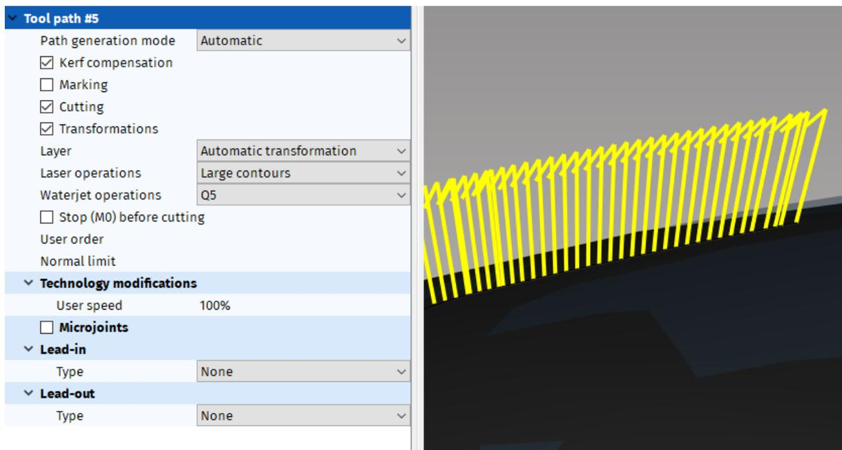
**Fig. 321: Lead-in none, lead-out none on gap cutting contour**
