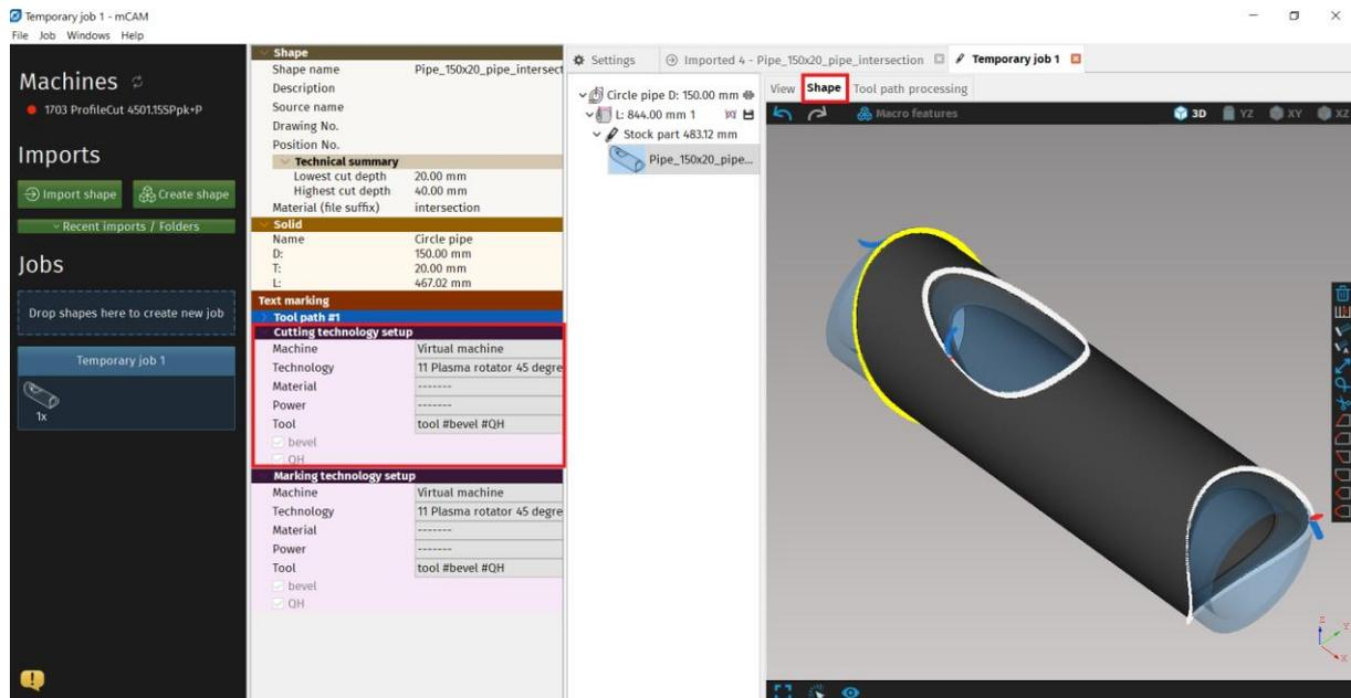
**Fig. 185: Plasma with respective tool is selected for text marking in Shape tab**
