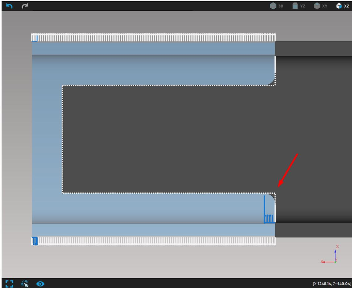
**Fig. 136: The model should be drawn without the radiuses**
