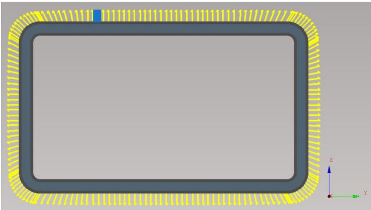
**Fig. 307: Cutting path – with pre-tilting in corners**
