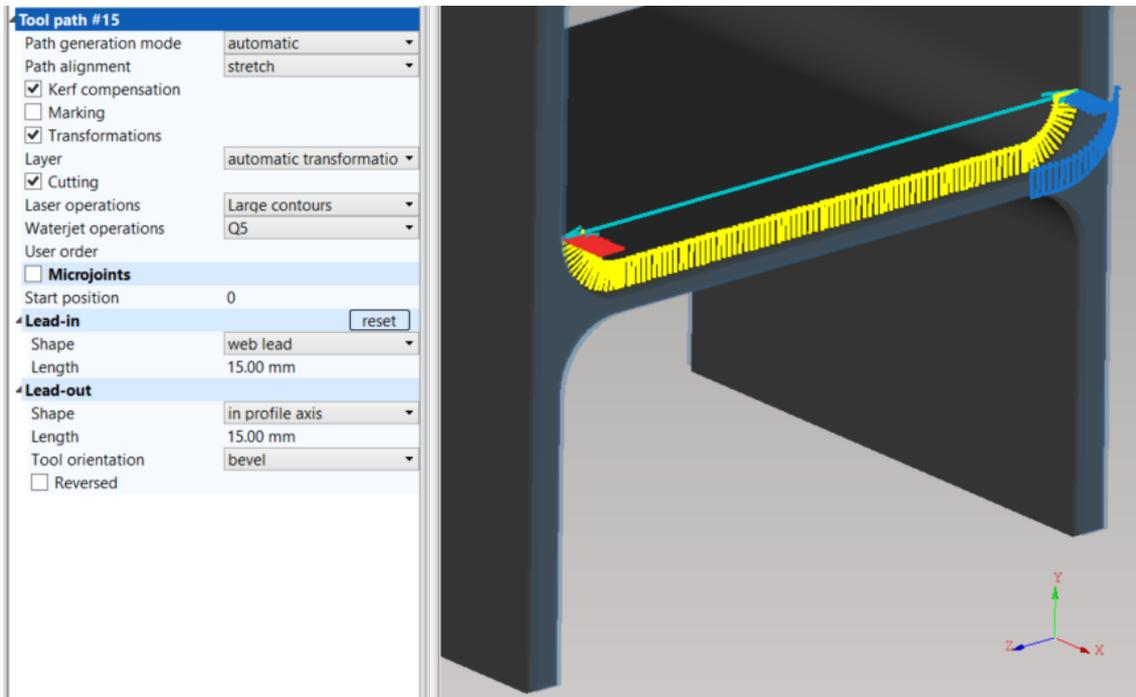
**Fig. 329: Lead-in Web lead, Lead-out in profile axis**
