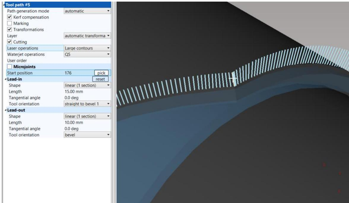
**Fig. 180: Selection of cutting point – start position**
