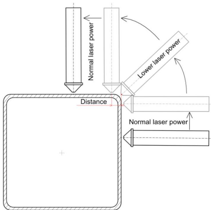
**Fig. 340: Affected area by reduced laser power**
