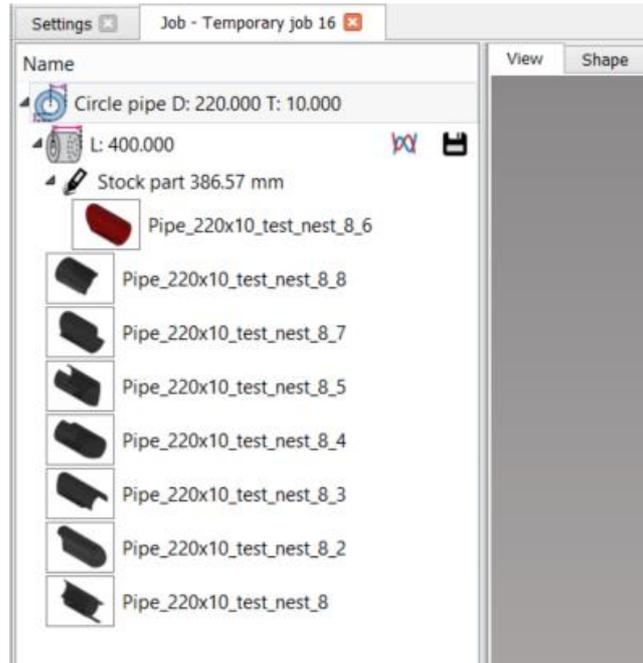
**Fig. 259: Unassigned or non-nested parts (grey parts)**
