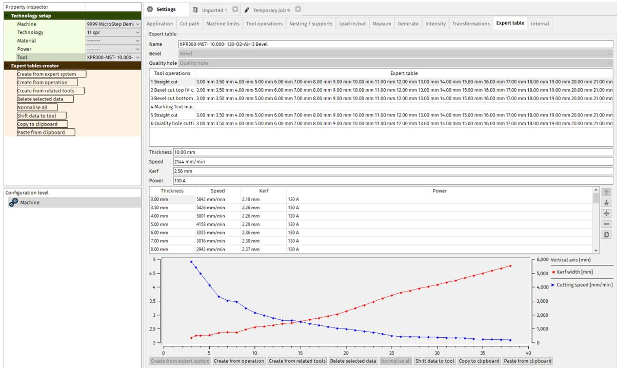
**Fig. 63: Expert cutting tables – cutting parameters (kerf width/cutting speed)**
