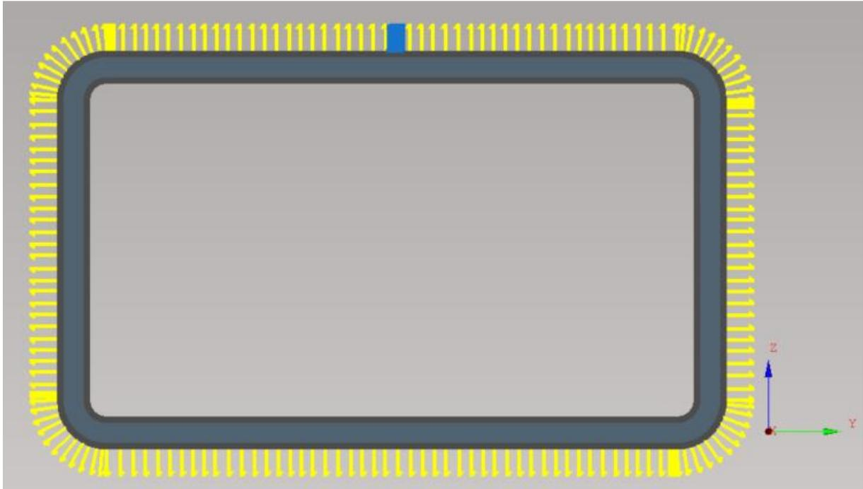
**Fig. 306: Cutting path – without pre-tilting in corners**
