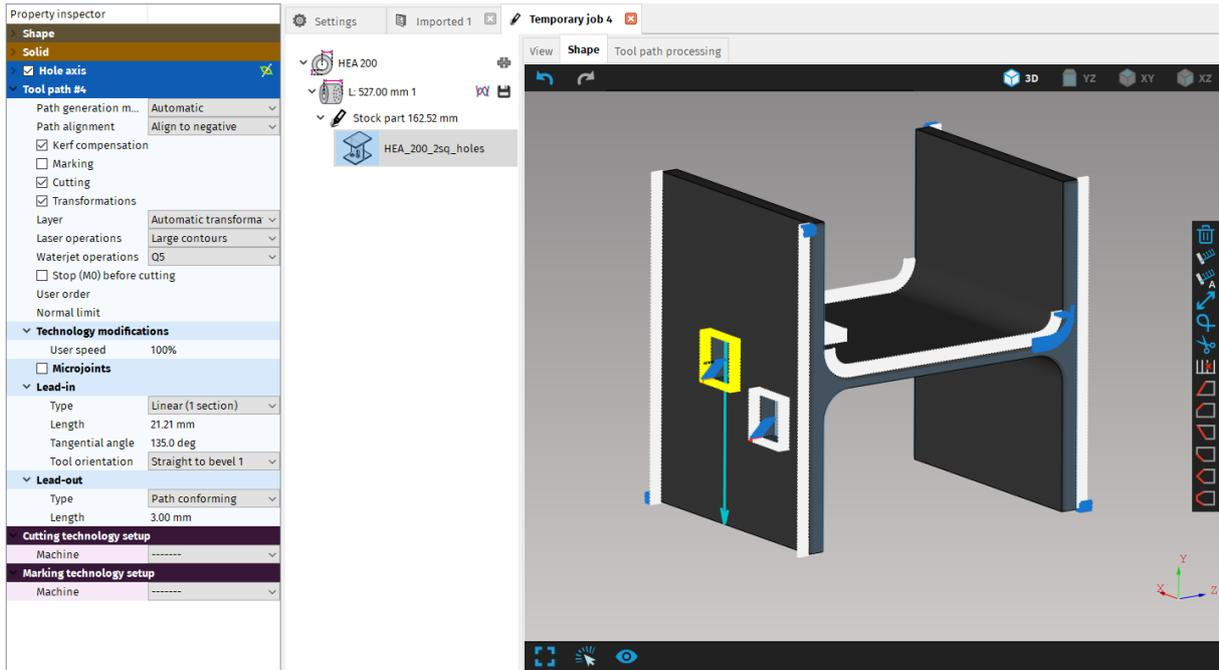
**Fig. 142: Align to negative – hole will maintain the distance from the bottom edge**
