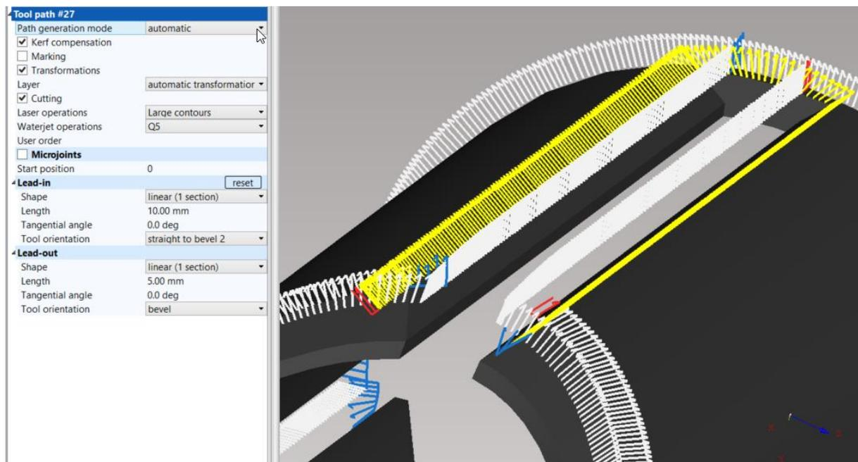
**Fig. 160: Complex surfaces and weld edge preparation – automatic mode**
