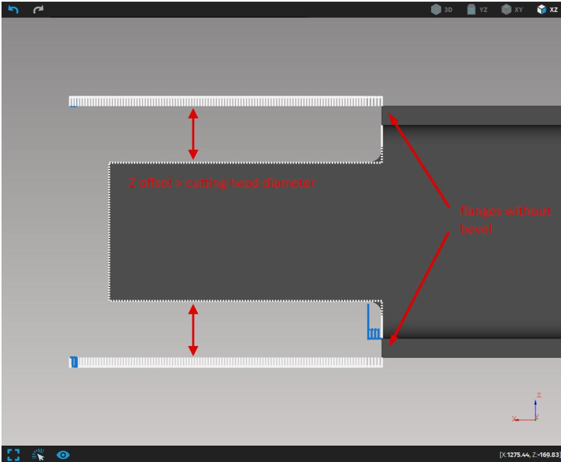
**Fig. 137: Cutting the tongue without using the macros**
