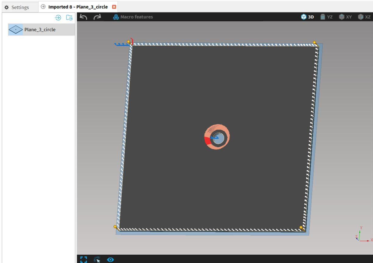
**Fig. 209: Automatic Welding preparation for Hole**
