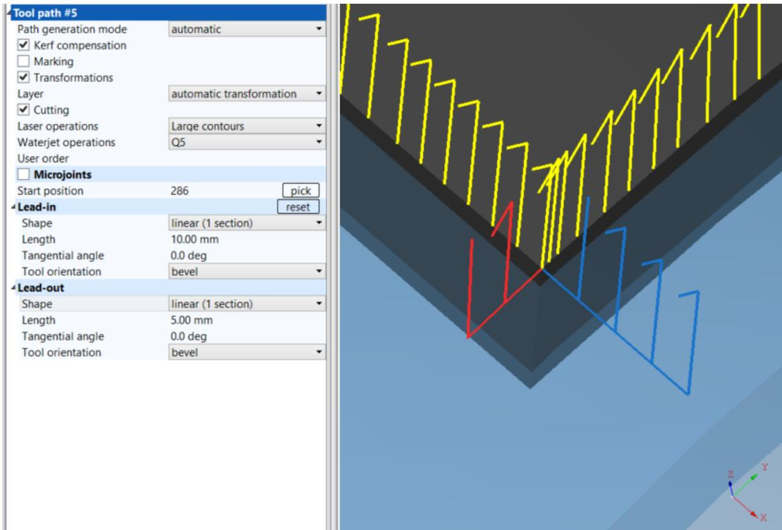
**Fig. 324: Lead-in linear (1 section), Lead-out linear (1 section)**
