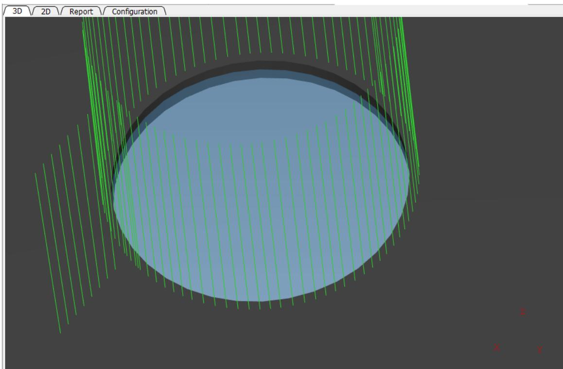
**Fig. 172: Kerf width compensation on the reversed cut path is on the outer side of the hole thus preserving the desired dimension of the final product.**
