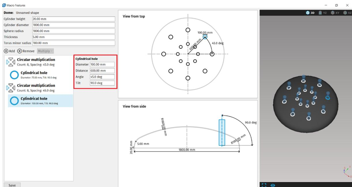
**Fig. 94: The properties of Cylindrical hole**
