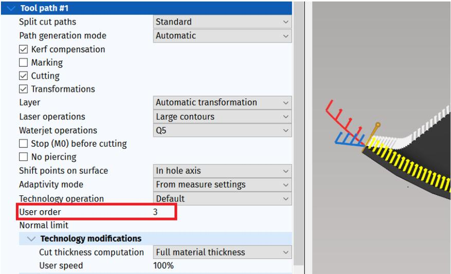
**Fig. 378: Setting the cutting order for each cutting path in mCAM**
