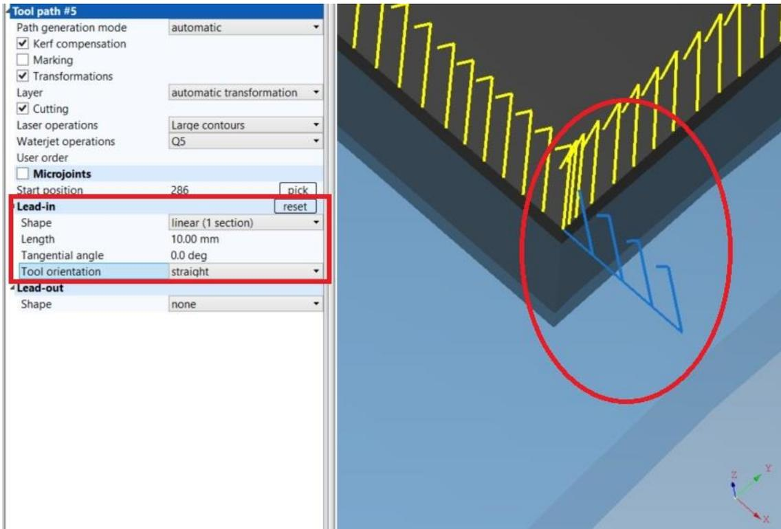
**Fig. 331: Tool orientation – straight (not suitable on bevel cuts)**
