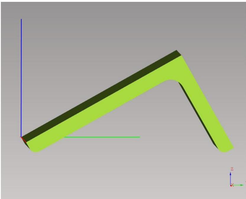
**Fig. 87: L-bar – shorter side has to be in Y+ direction**
