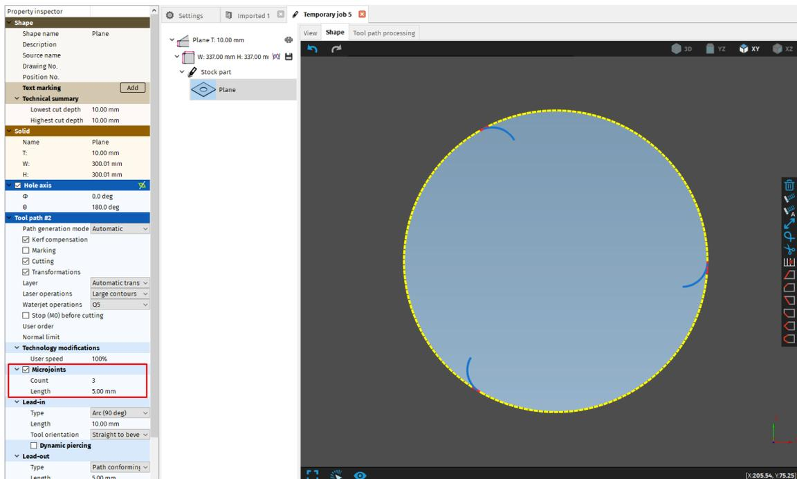
**Fig. 236: Using microjoints to split path to three smaller fragments.**
