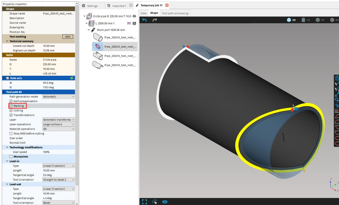
**Fig. 274: Cutting path properties – marking enabled**
