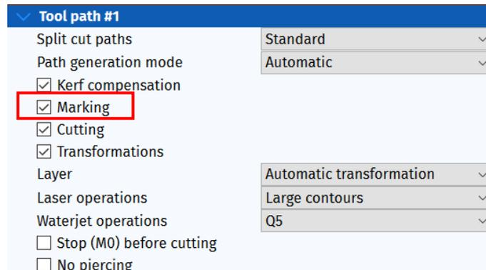
**Fig. 380: Marking checkbox in mCAM**
