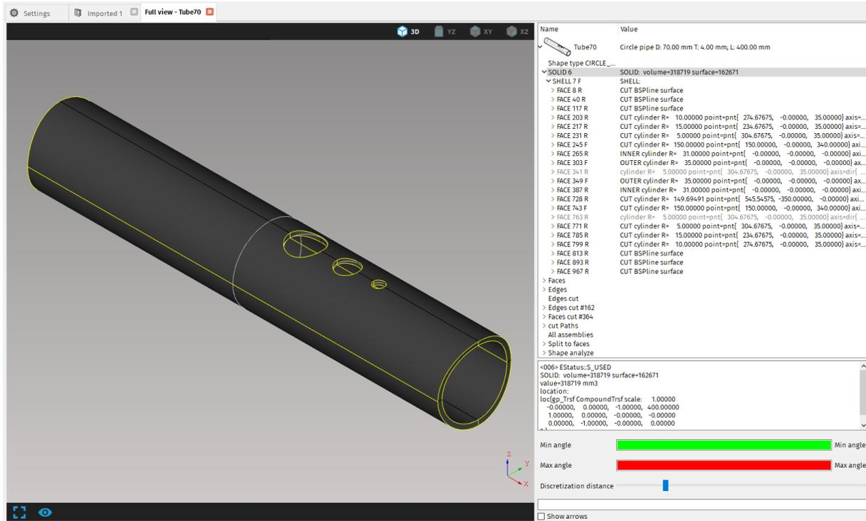
**Fig. 352: Geometrical structure of 3D solid (B-rep model)**
