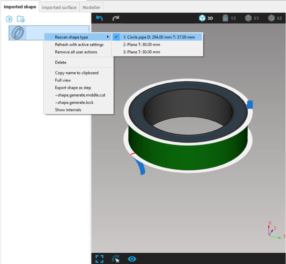
Fig. 349: Rescan shape type to Circle pipe
