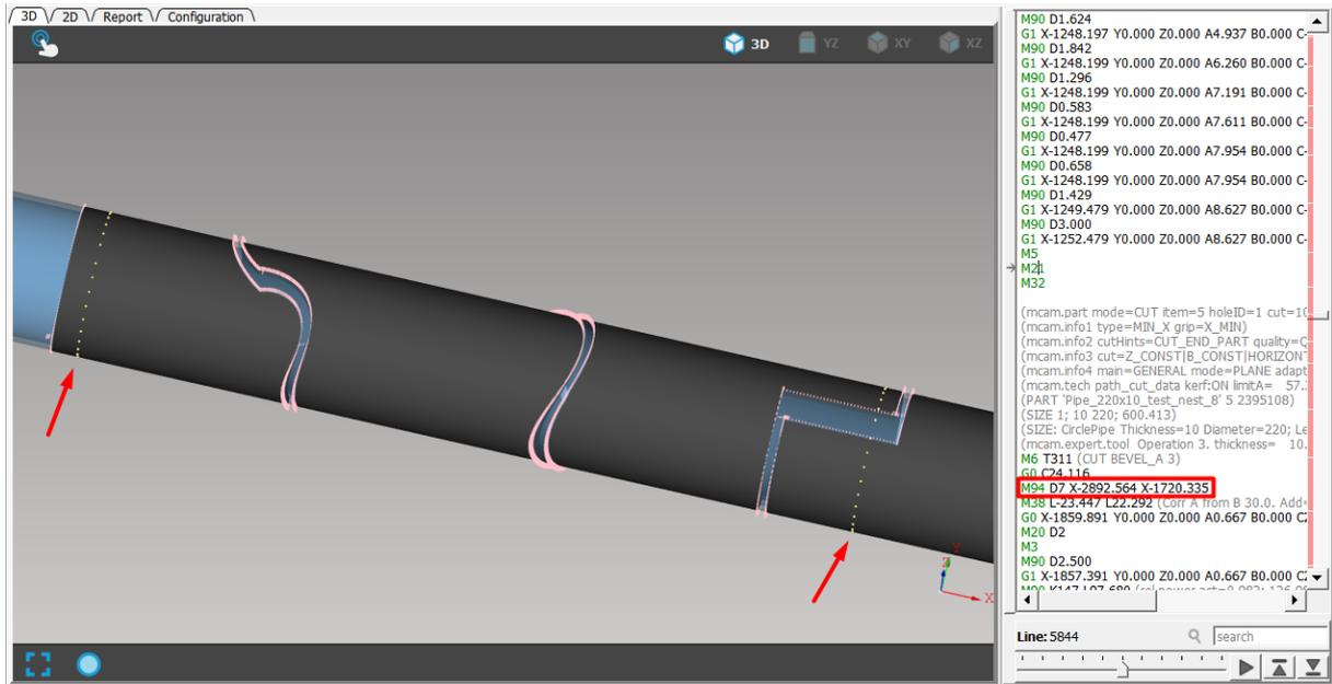
**Fig. 335: Measuring on two X positions for group of cuts on pipe**
