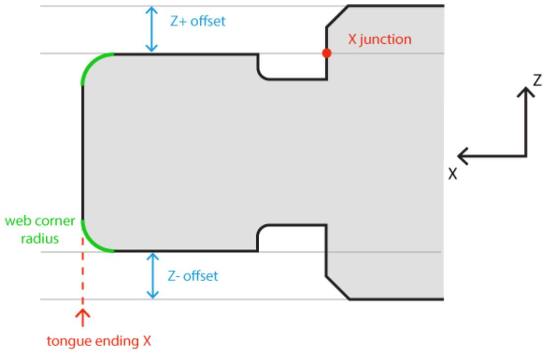
**Fig. 122: Parameters for Tongue ending welding connection**
