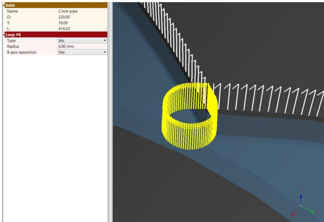
**Fig. 177: Loop type – arc**
