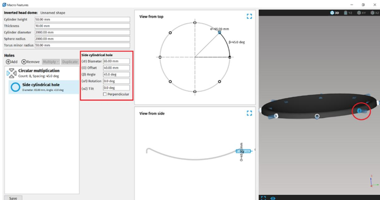
**Fig. 113: Example of Side cylindrical hole macro placed on Inverted head dome**
