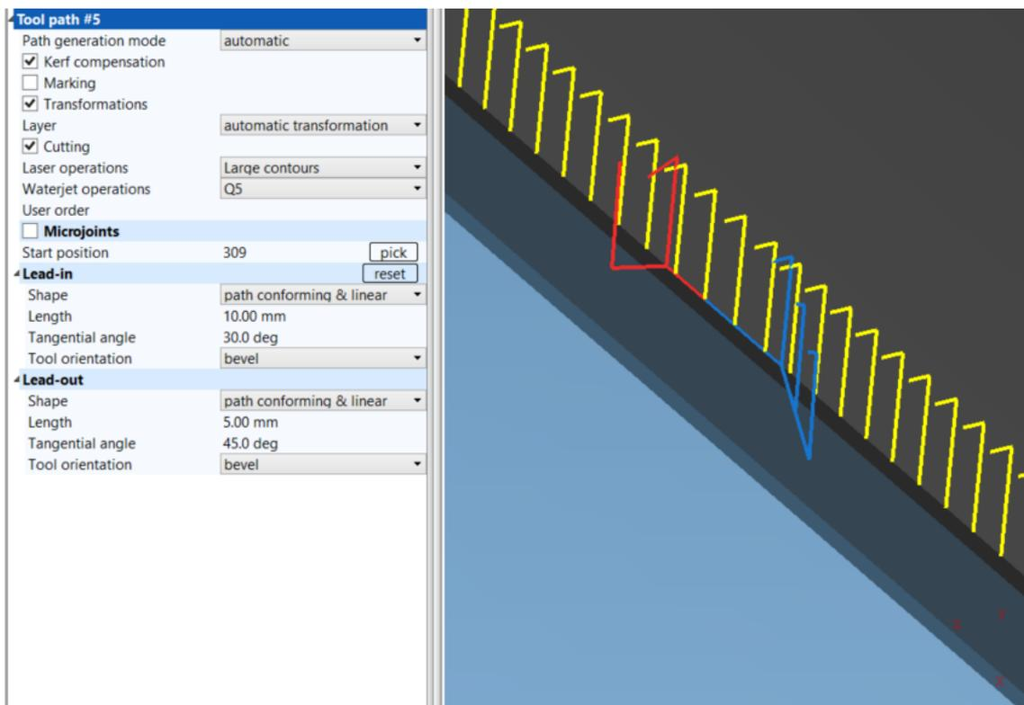
**Fig. 323: Lead-in path conforming & linear, Lead-out path conforming & linear**
