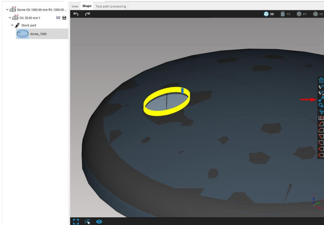
**Fig. 169: Reversing cut path button in the cut path editing widget**
