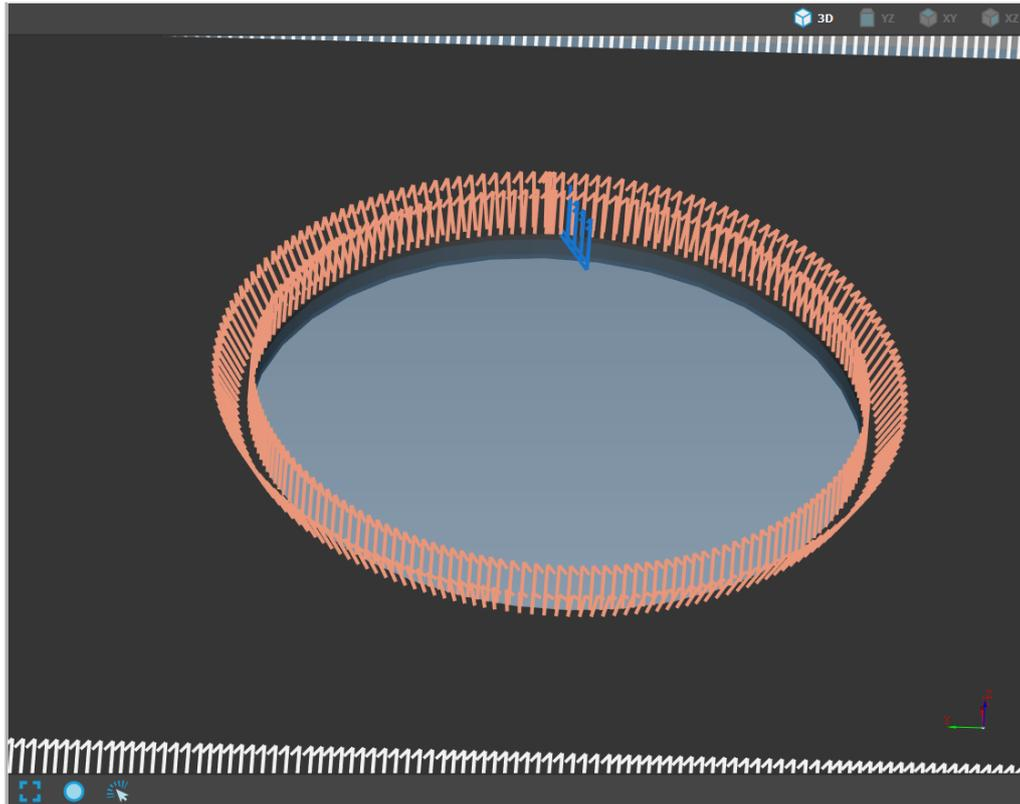
**Fig. 204: Hole with Y welding preparation**
