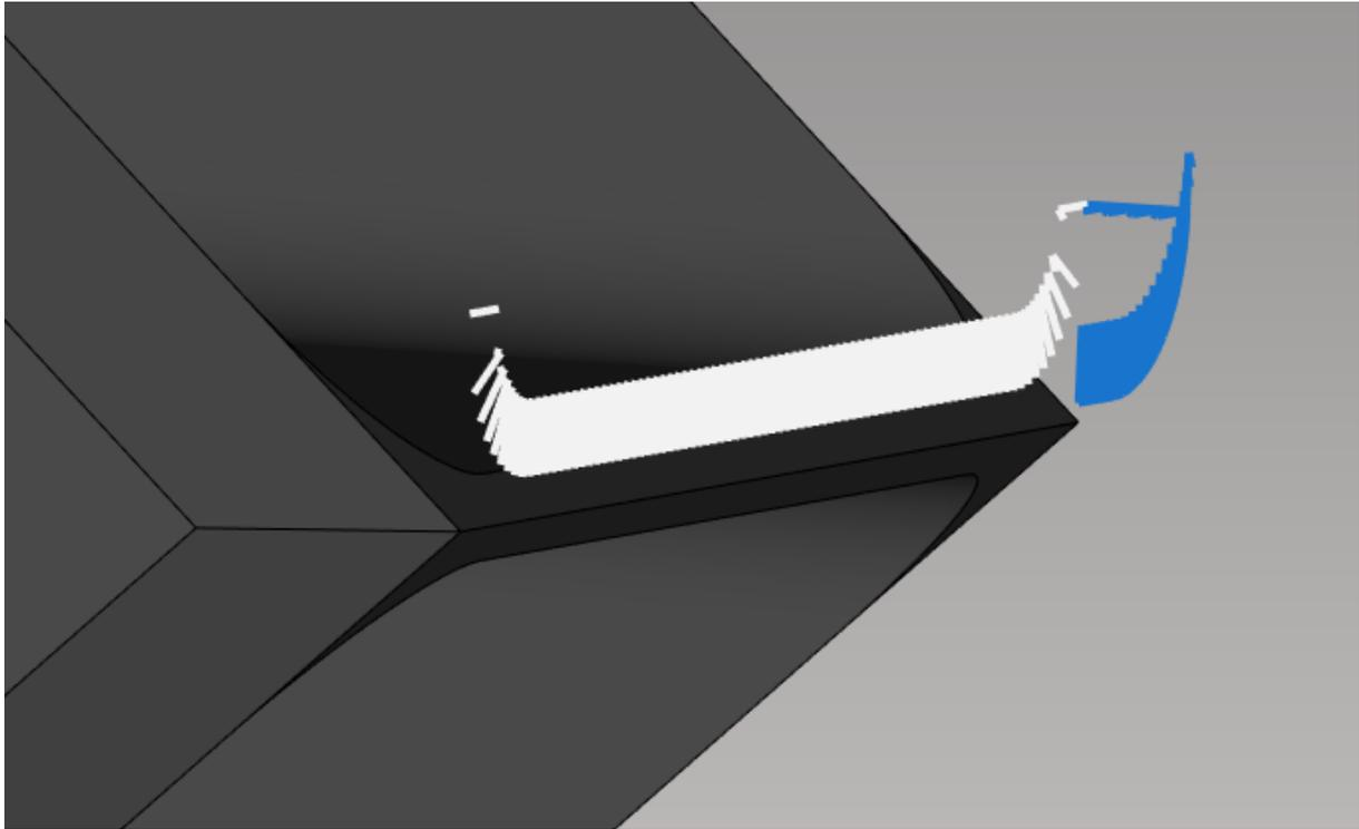
*Fig. 132: Step file is designed with X cut on the web, but the final cut is straight*
