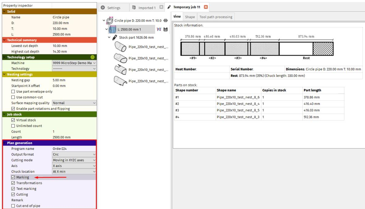
**Fig. 275: Stock properties and plan generation options**
