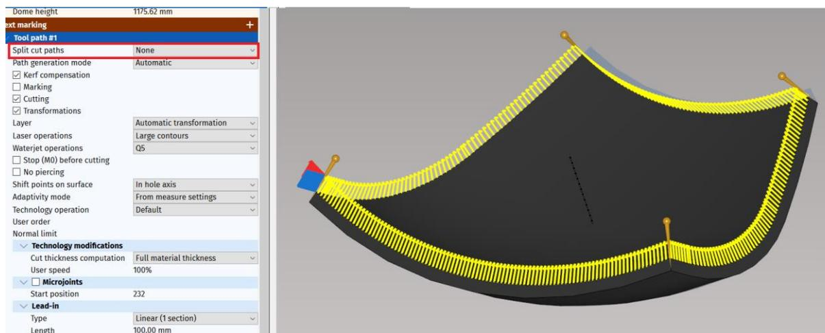
**Fig. 375: Cut paths before splitting in mCAM**
