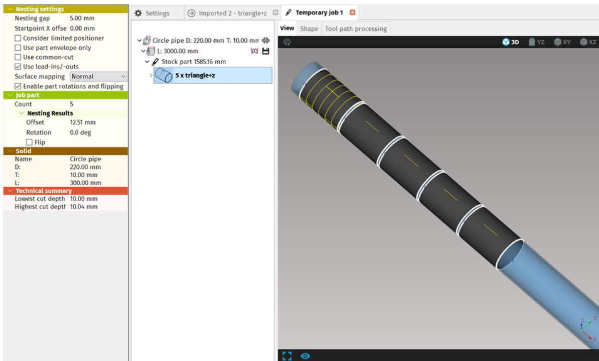
**Fig. 213: Nesting of circle pipe with welding line**
