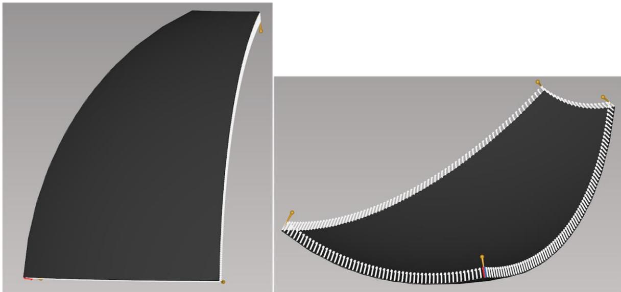
*Fig. 368: Spherical dome petal*
