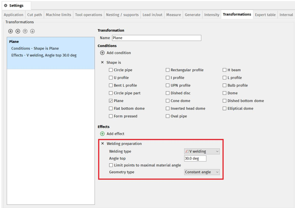
**Fig. 207: Further customization of Welding preparation**
