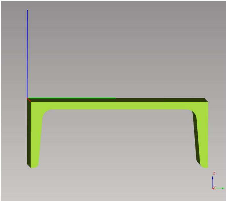
**Fig. 85: UPN-bar – Flanges are in Z-axis, with web facing Z+ direction**
