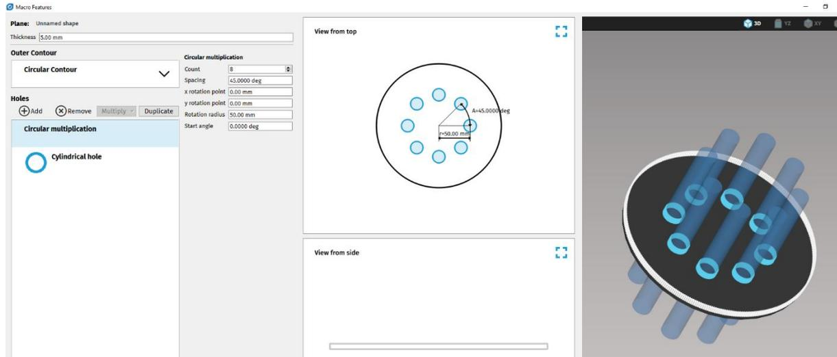
Fig. 114: Example of cylindrical hole macro placed on circular plane profile
