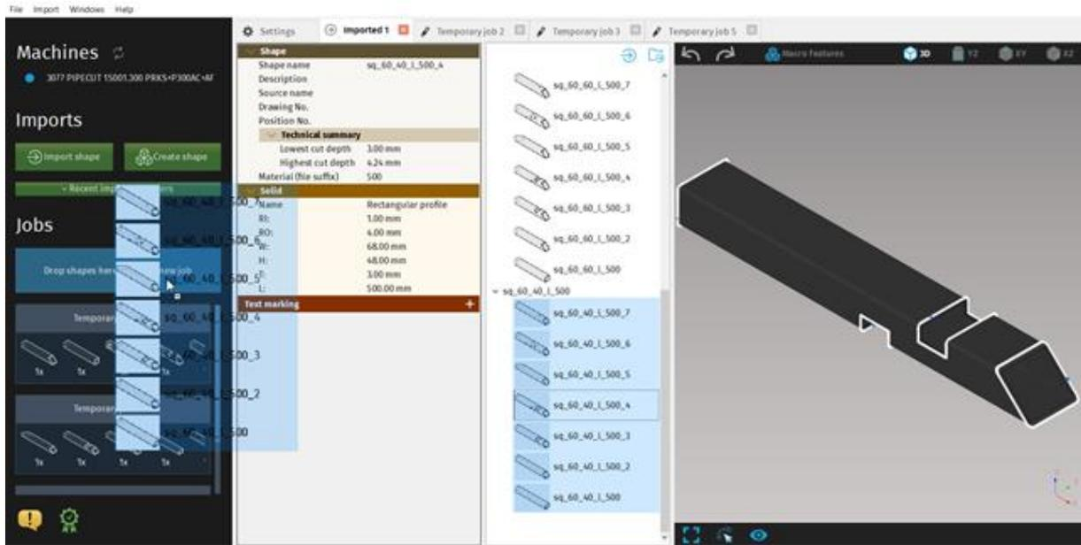
**Fig. 391: Drag shapes to create a new job in mCAM**
