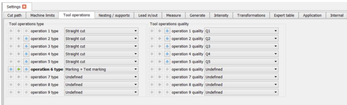
**Fig. 198: Standard water – jet tool operations setup**
