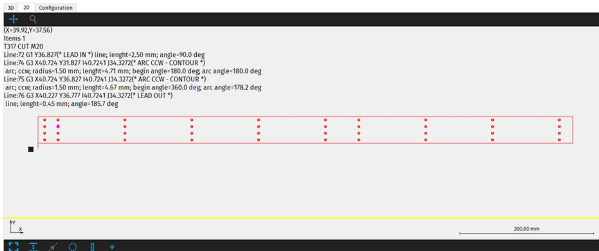
**Fig. 286: Tooltip information in mCAM simulation**
