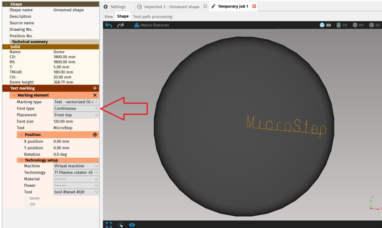
**Fig. 194: Font type in Text marking section of Properties menu**
