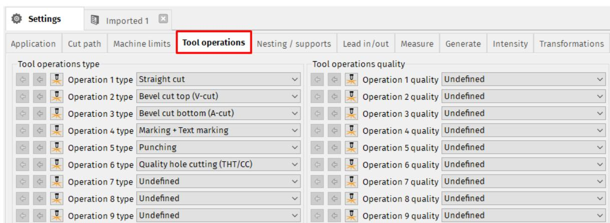
**Fig. 311: Tool operation settings – tools**
