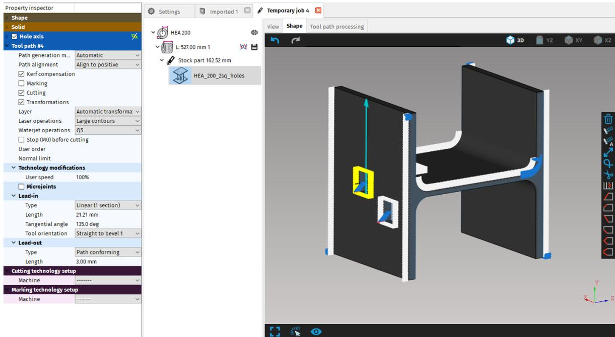
**Fig. 140: Align to positive – hole will maintain the distance from the top edge**
