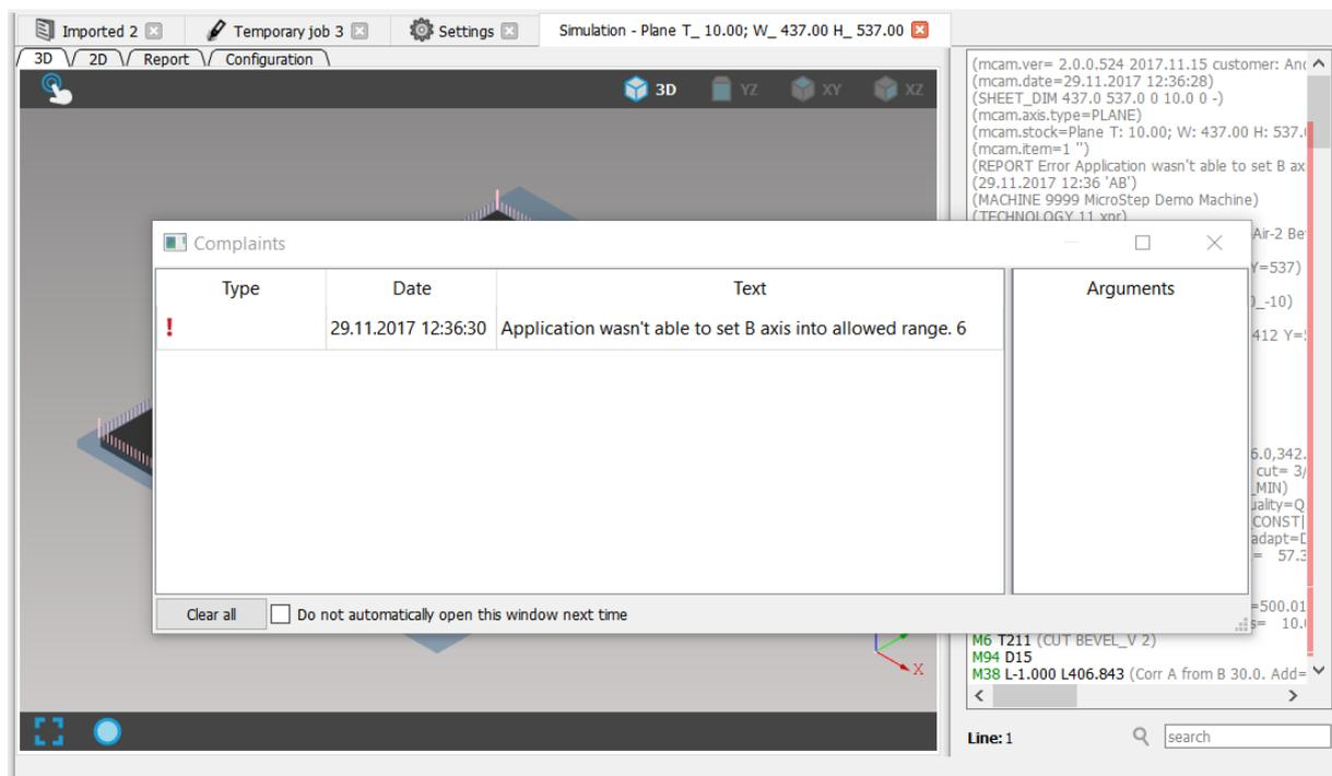
**Fig. 234: Complaint about exceeded range of B-axis**
