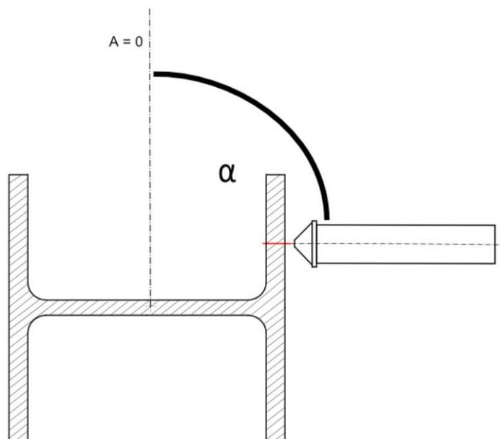
**Fig. 309: Maximum A axis angle for cutting and marking**
