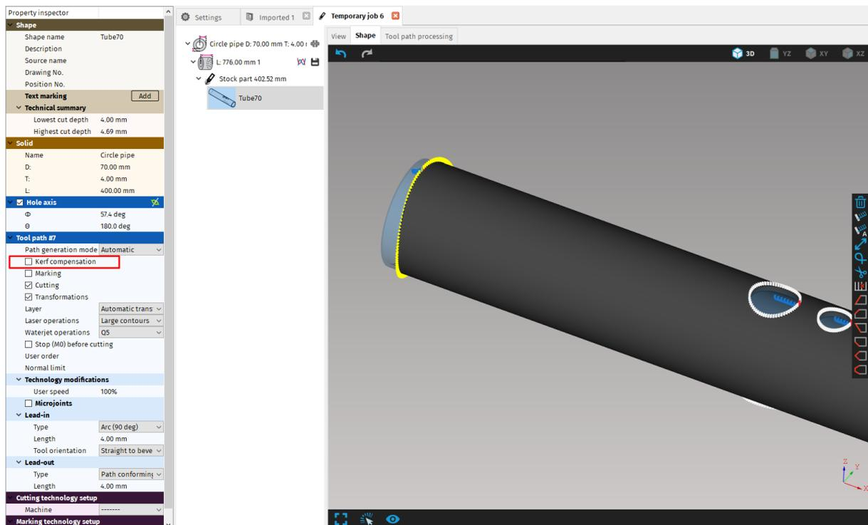
**Fig. 244: Disabling kerf width compensation on selected cutting path**
