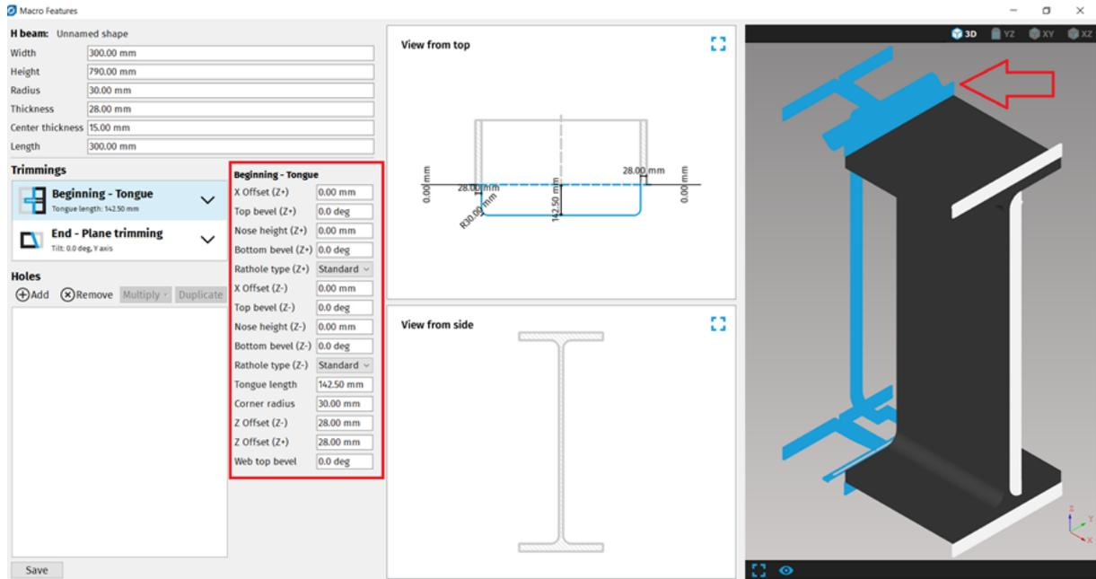
**Fig. 107: Example of a Tongue in Trimmings for H beam**
