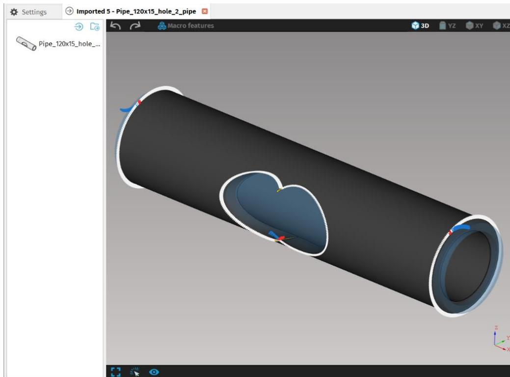
**Fig. 2: Imported circular pipe from STEP file**
