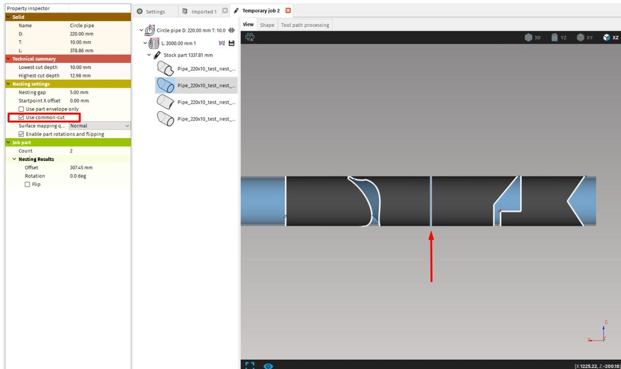
**Fig. 255: Applied common-cut**
