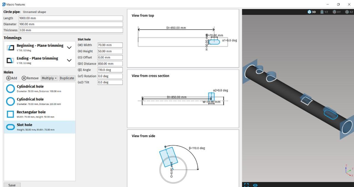
**Fig. 4 Examples of macros for Circular pipe in Macro feature**
