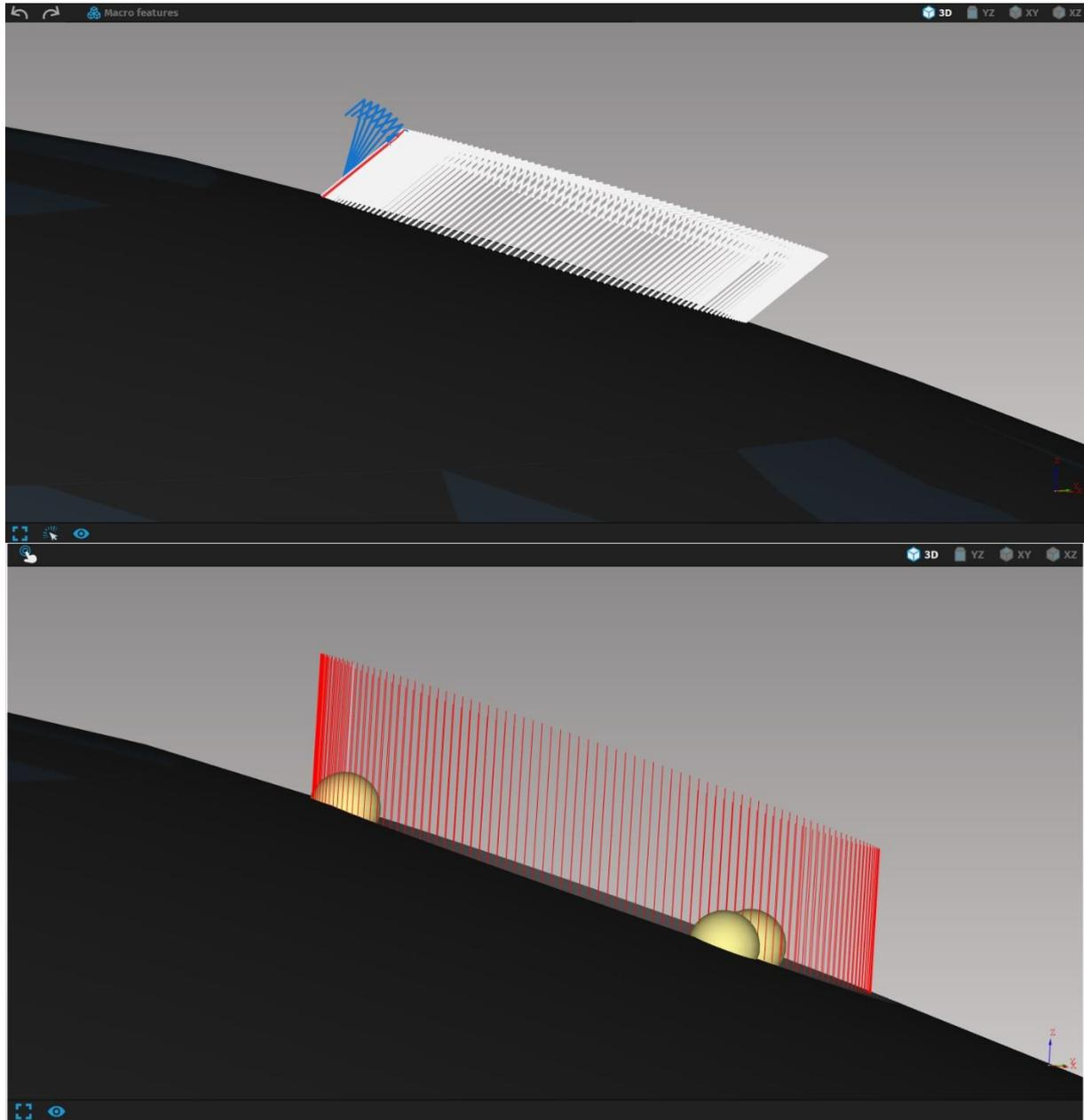
**Fig. 281: A-axis hardware limitation before the simulation and after the limitation in simulation with 0° maximum tilt cutting head**
