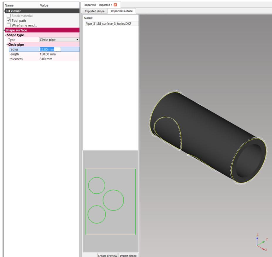
**Fig. 45: Parametrized 3D shape (import 2D surface – \*.dxf)**
