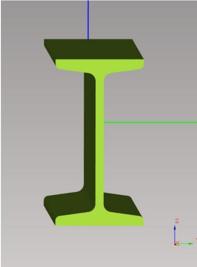
**Fig. 80: I-bar – (older position) top edge of cutting contour, where the cutting starts, needs to be in Y+ direction**
