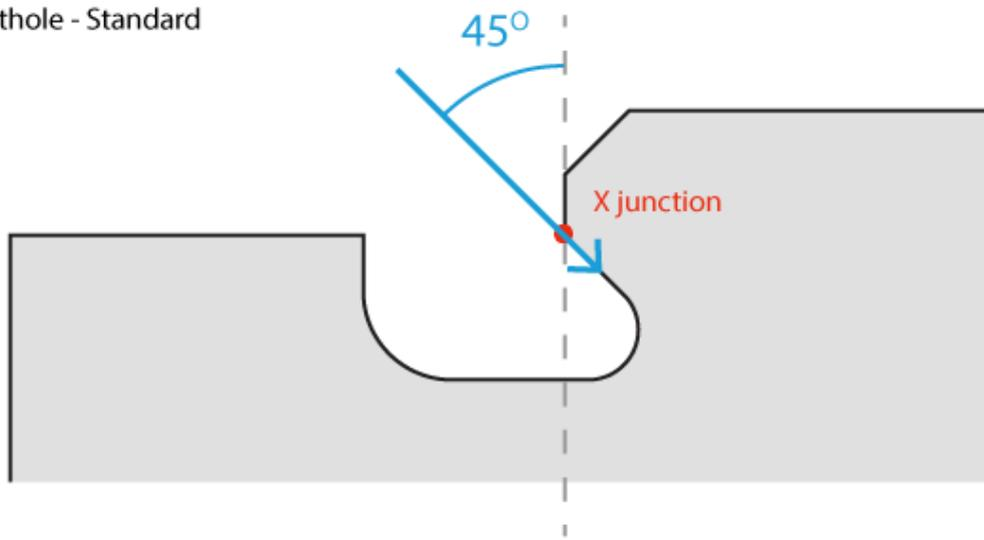
**Fig. 124: Rathole Standard is cut in 45 degrees angle**
