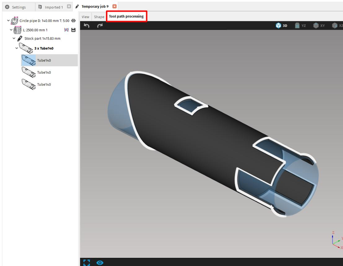
**Fig. 65: Tool path processing – limited and compensated according to set machine and tool**
