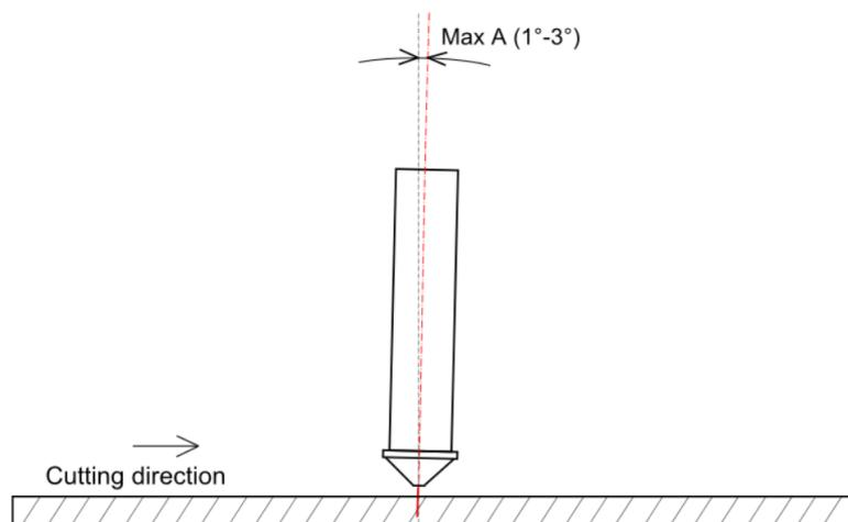
**Fig. 337: Maximum A axis angle for straight cut and for B-axis repositioning**
