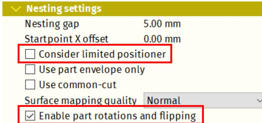
**Fig. 401: Consider Limited positioner option in Nesting settings in mCAM**
