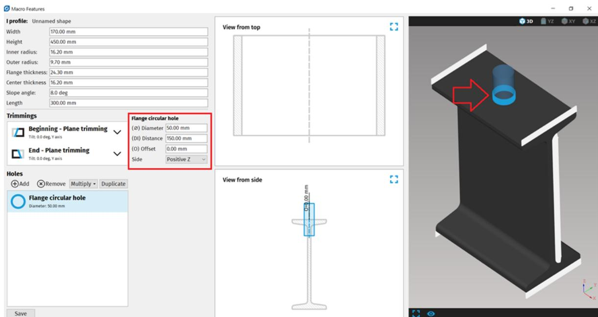
**Fig. 108: Example of Flange circular hole macro placed on I beam**
