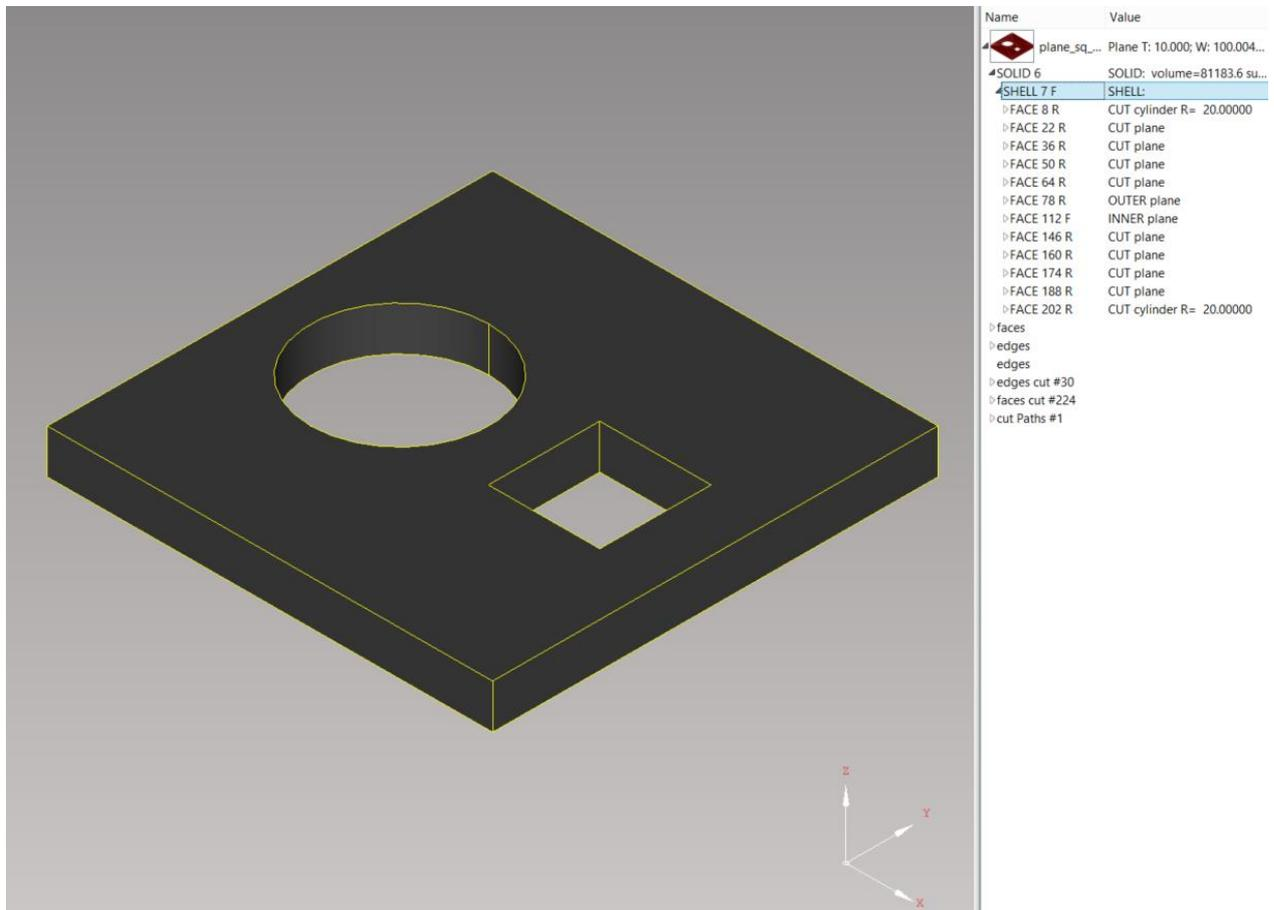
**Fig. 5: B–rep model using 12 faces**
