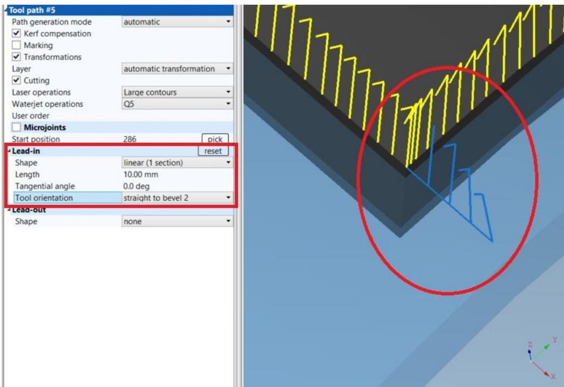
**Fig. 332: Tool orientation – straight to bevel 2**
