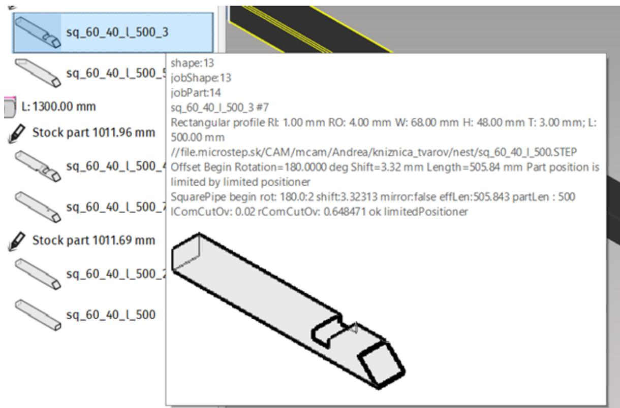
**Fig. 407: Nesting results shown in a tooltip**
