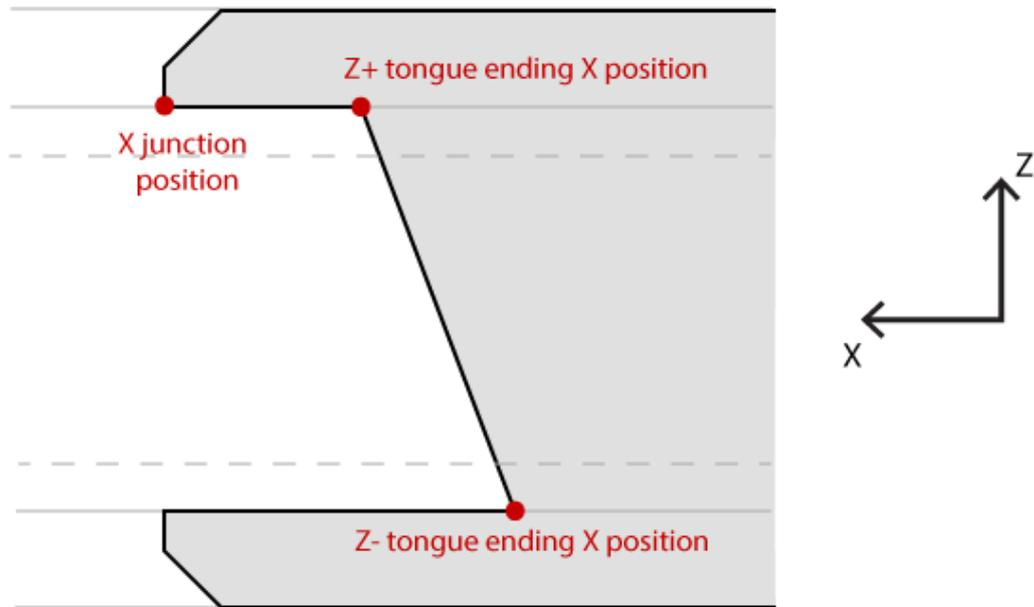
**Fig. 129: Inverse tongue ending with parameters**
