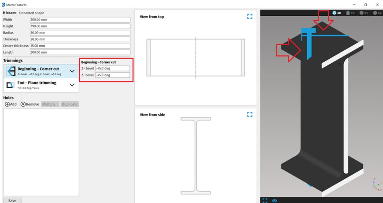
**Fig. 106: Example of Beginning – Corner cut in Trimmings for H beam**
