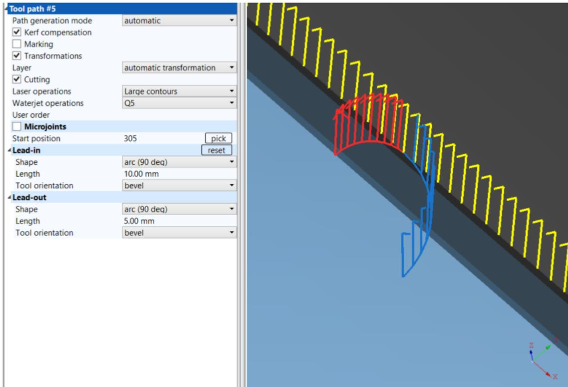
**Fig. 326: Lead-in arc (90 deg), Lead-out arc (90 deg)**
