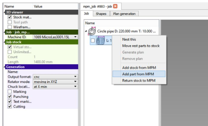
Fig. 365: Add parts from MPM database
