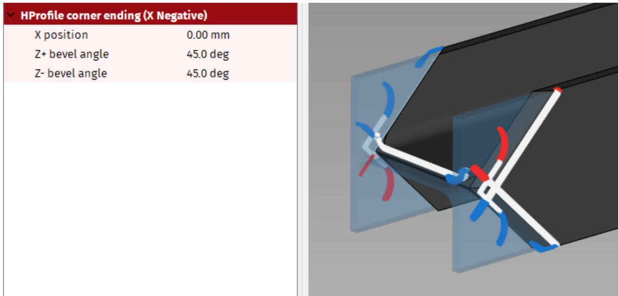
**Fig. 130: Corner ending and its parameters in Properties area**
