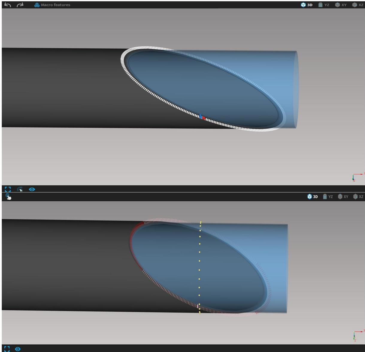
**Fig. 282: Limitation of machine angle between tool and material surface before and after the limitation in simulation**
