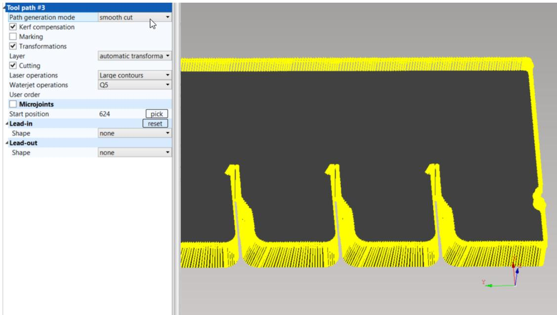
**Fig. 161: Complex cutting surfaces – planar shapes – smooth cut mode**
