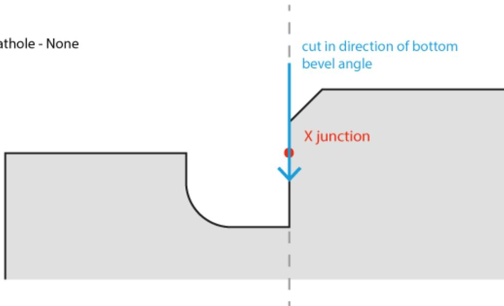
**Fig. 125: Rathole None is cut in direction of bottom bevel angle**
