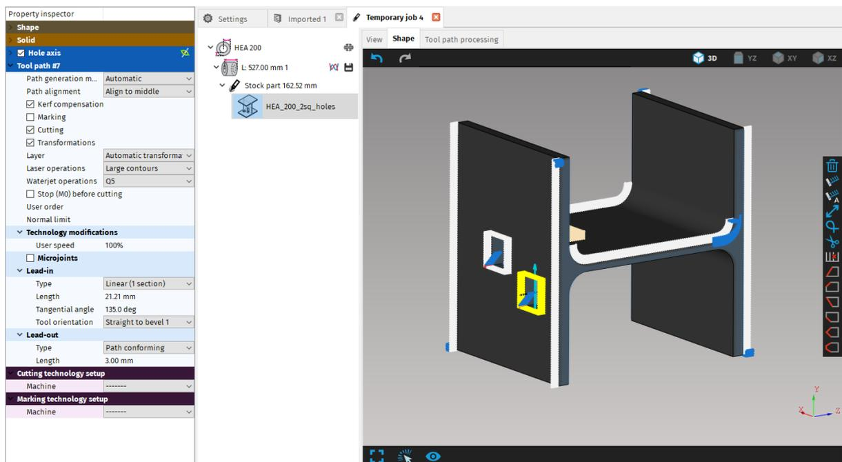
**Fig. 141: Align to middle – hole will maintain the distance from the middle of flange**
