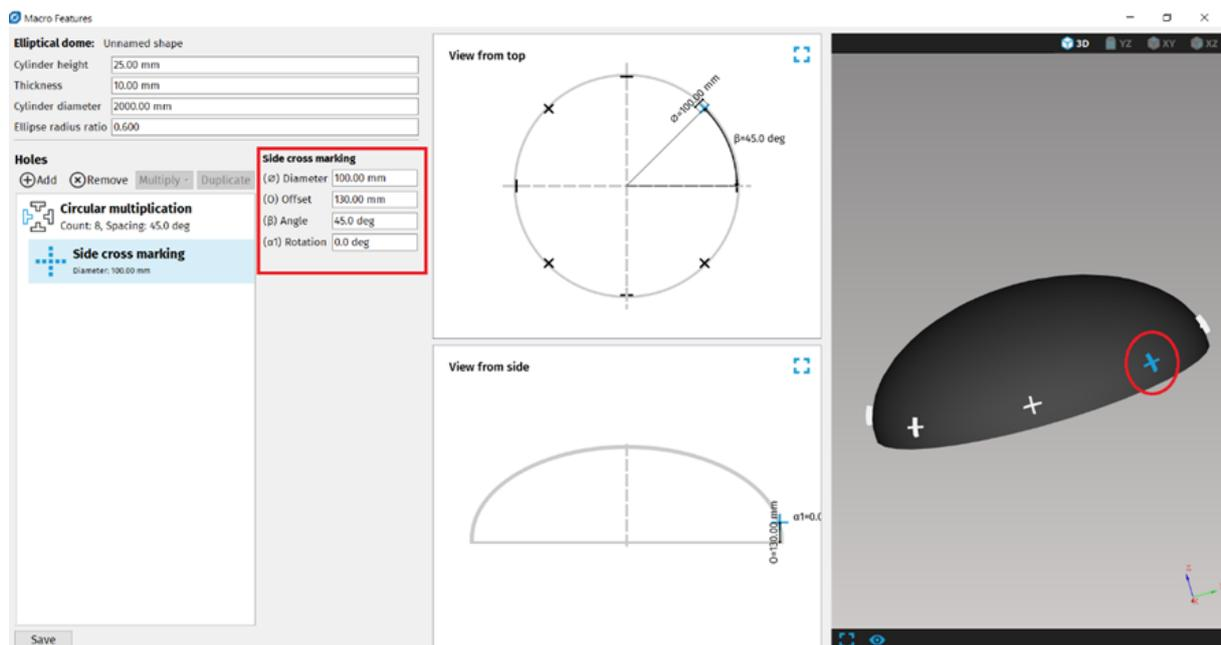
**Fig. 111: Example of Side cross marking macro placed on Elliptical dome**
