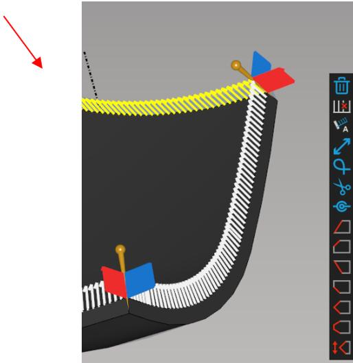
**Fig. 379: Deleting the selected cutting path in mCAM**
