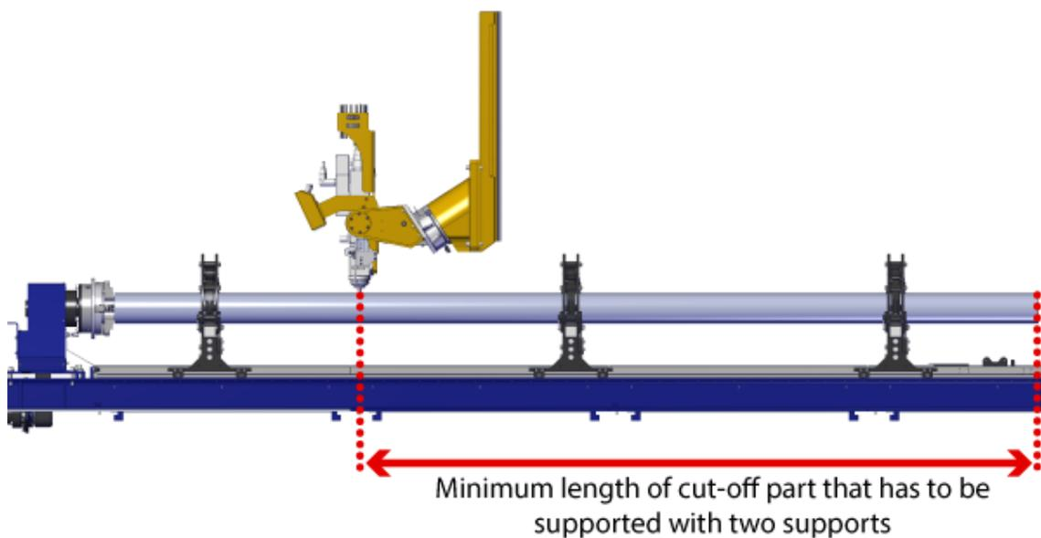
**Fig. 317: Min length of the cut-off part to be supported with two supports**
