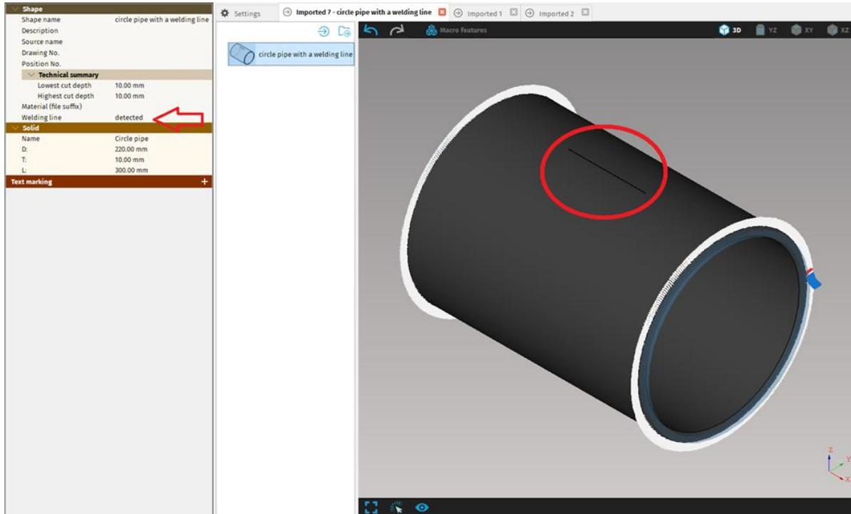
**Fig. 212 Circle pipe with groove marking the welding line**
