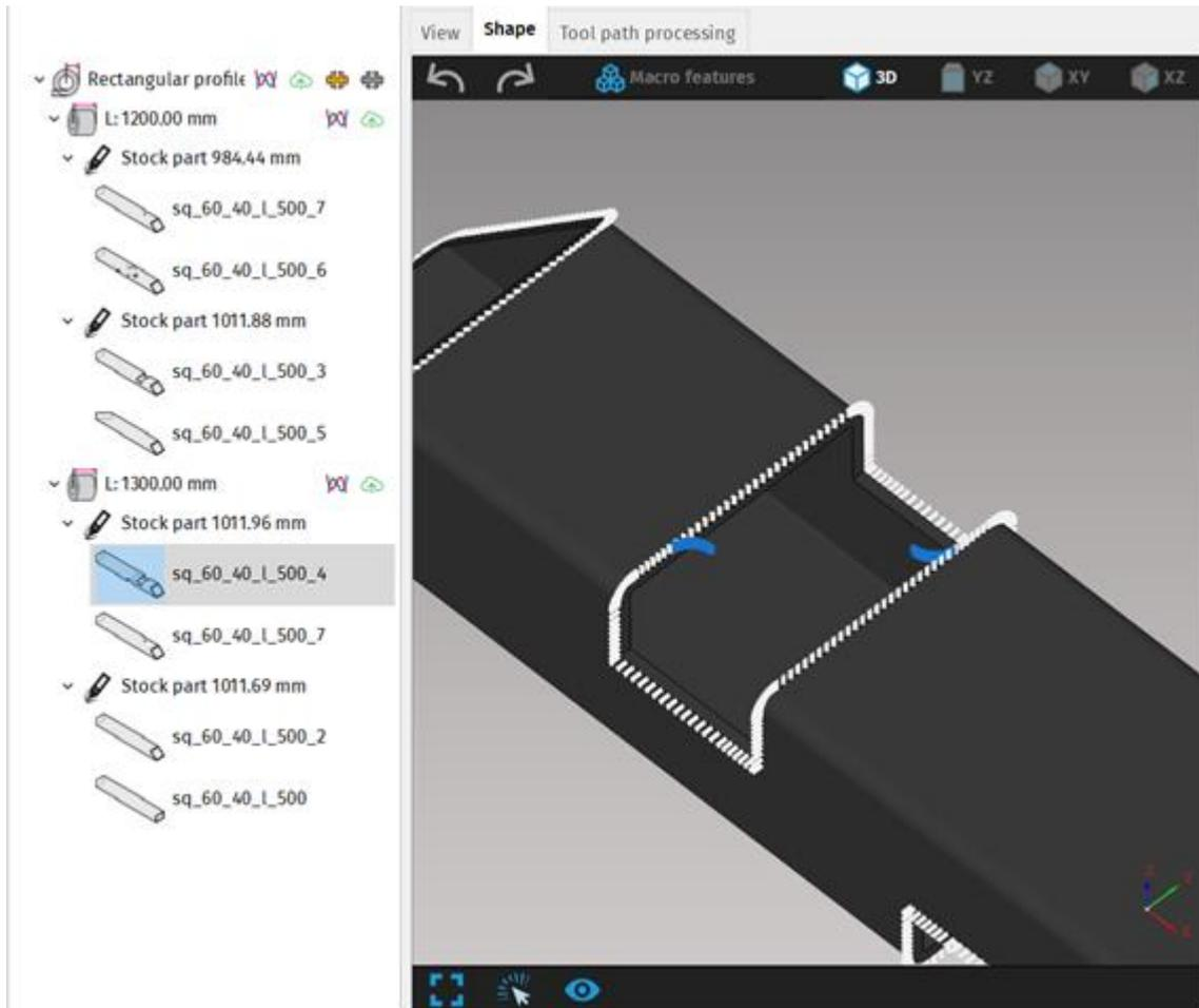
**Fig. 403: Microjoints applied to cut**
