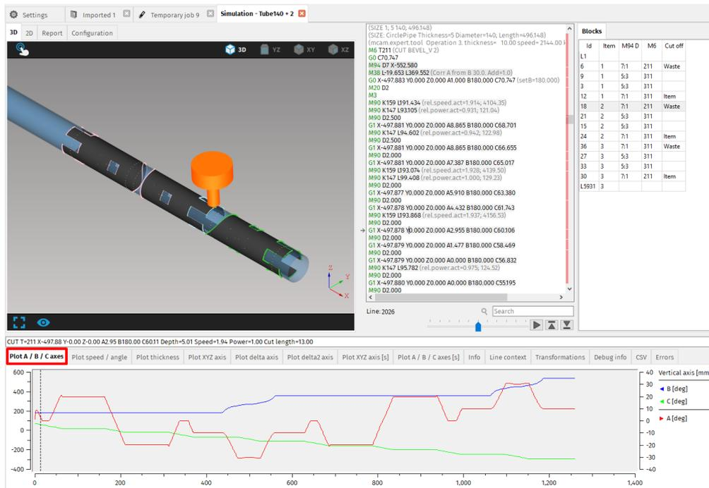
**Fig. 67: Cutting simulation and plotting A, B and C axes movements**
