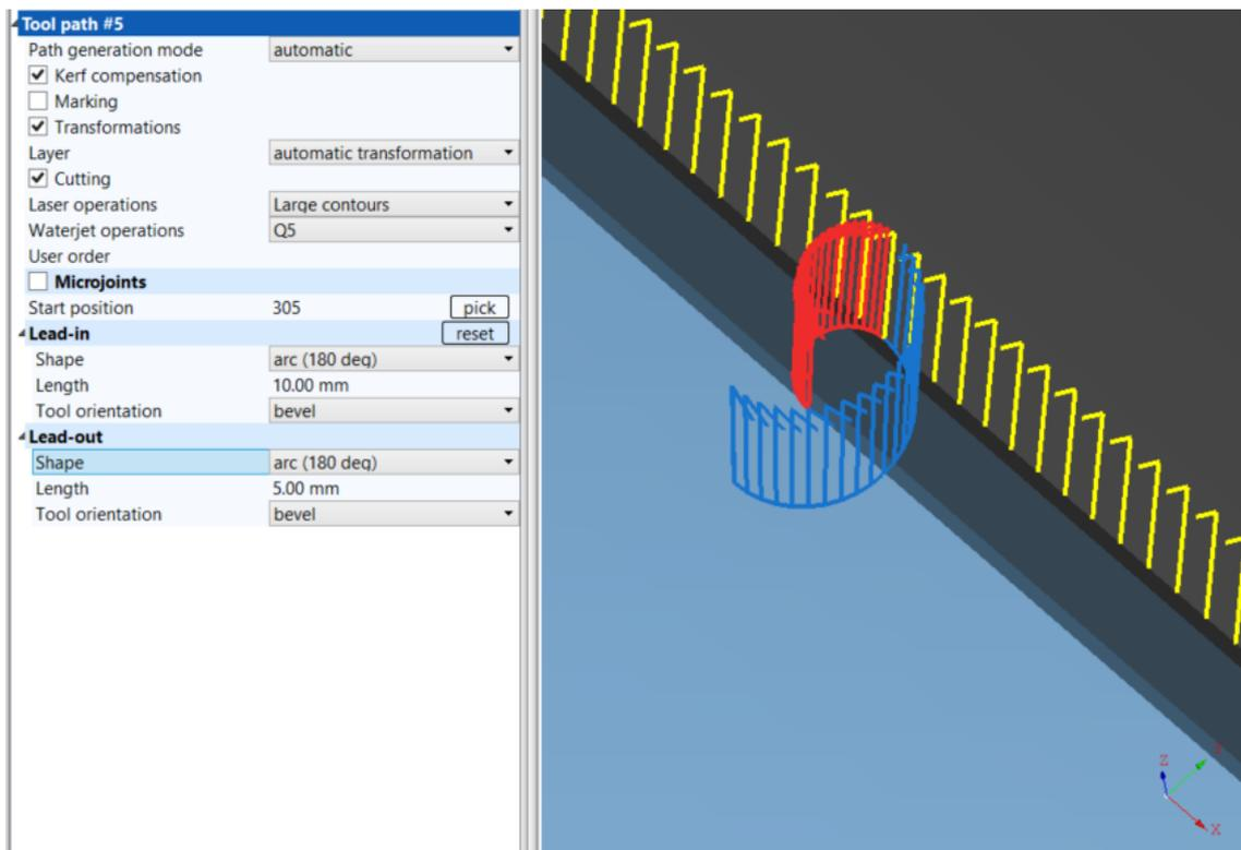
**Fig. 327: Lead-in arc (180 deg), Lead-out arc (180 deg)**
