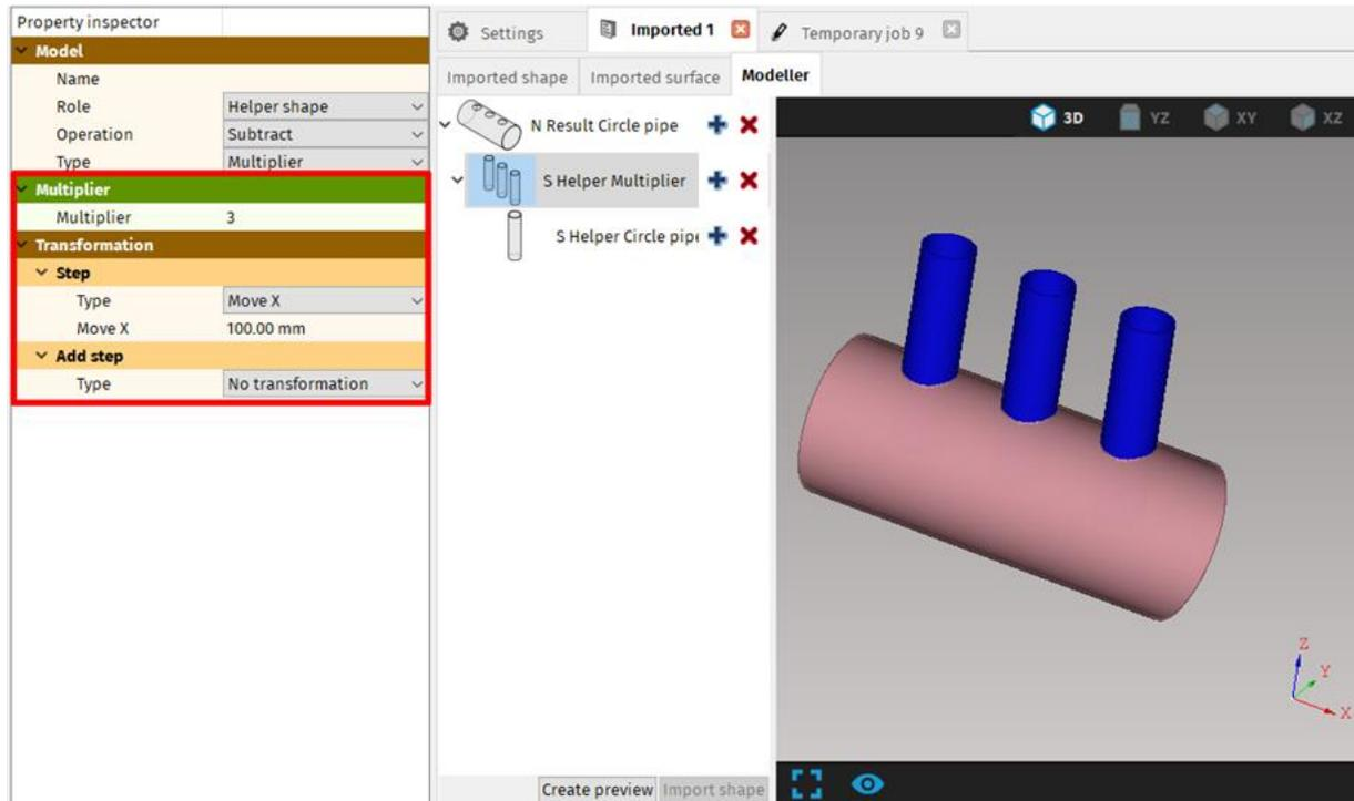
**Fig. 89: Three circle pipes spaced out across the result shape by 120mm**
