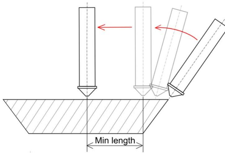
**Fig. 302: Minimal length for torch shifting to material normal on planar surface**
