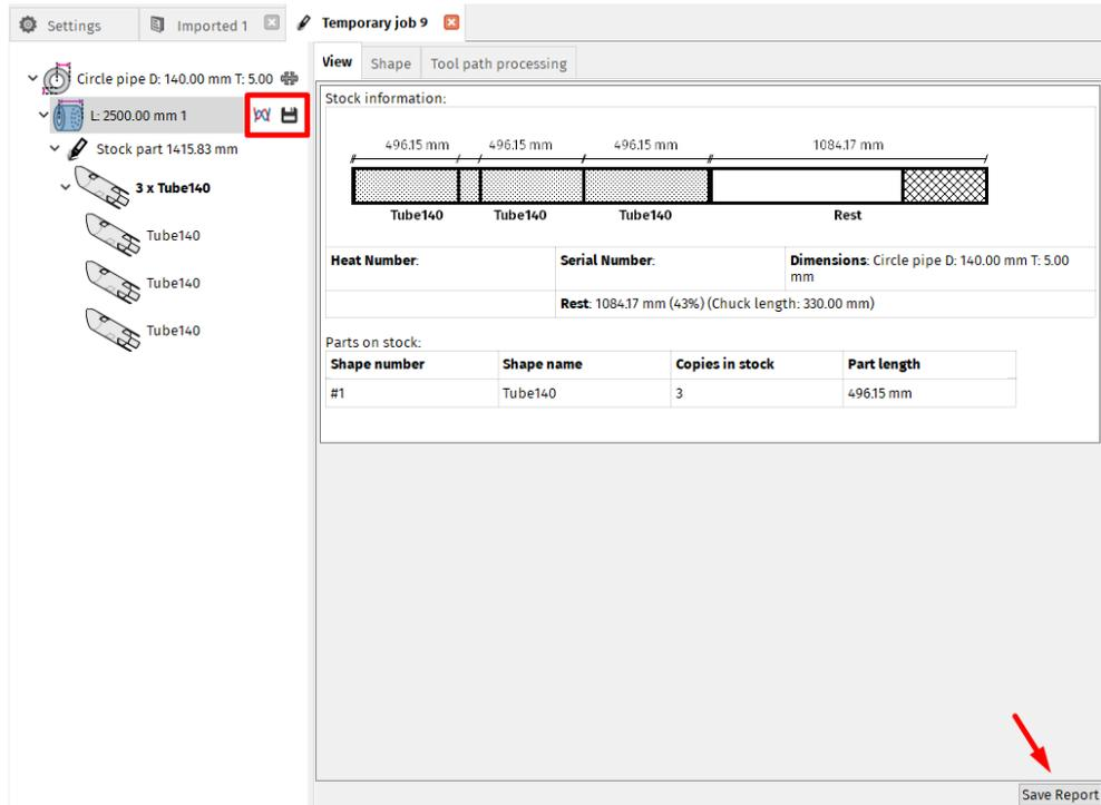
**Fig. 66: Cutting simulation, saving CNC plan to the right of selected stock, saving nesting report in pdf. file in the bottom right corner**
