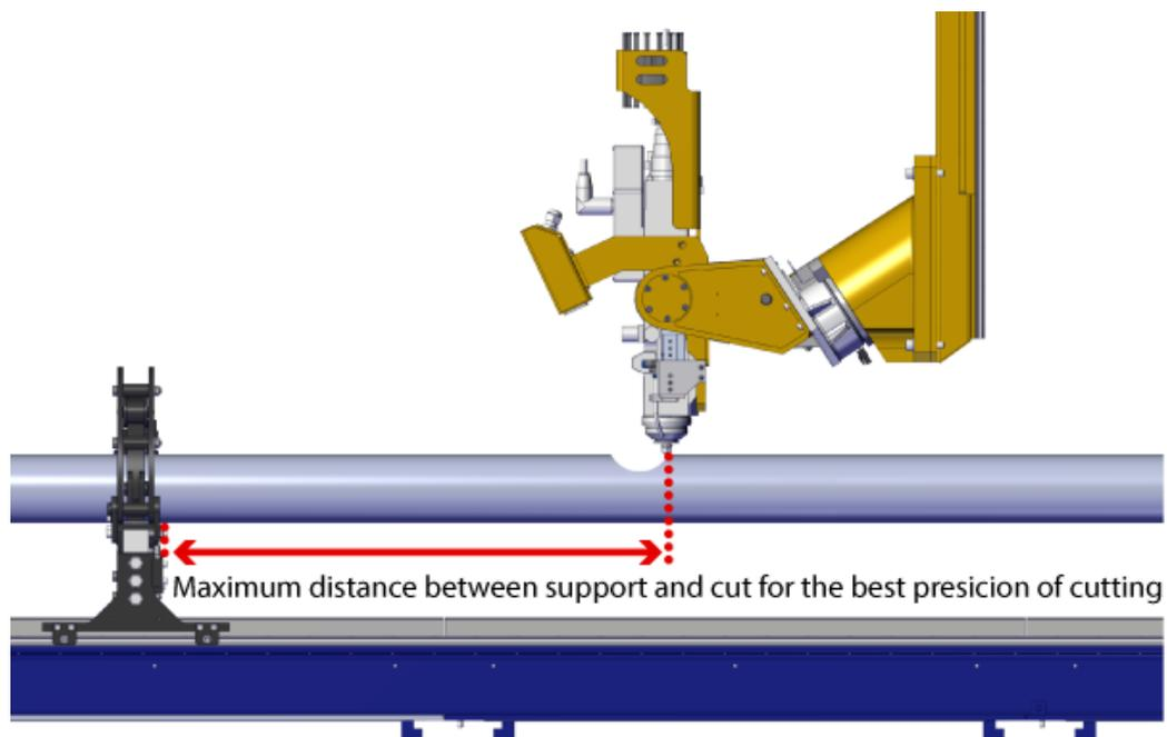
**Fig. 316: Maximum support-cut distance**
