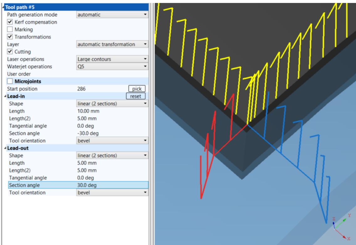
**Fig. 325: Lead-in linear (2 section), Lead-out linear (2 section)**
