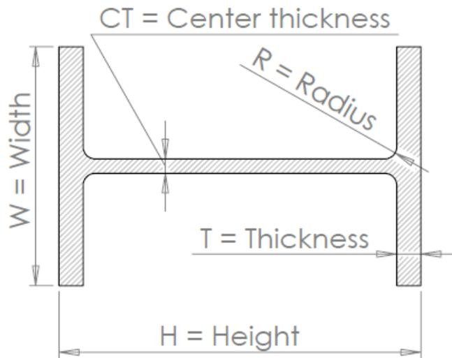
**Fig. 13: H Beam - HEA, HEB, HEM and IPE beams (parallel flanges)**
