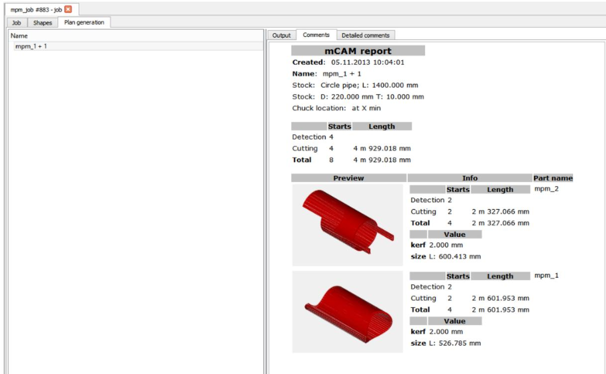
**Fig. 367: Report of generated cutting plan**
