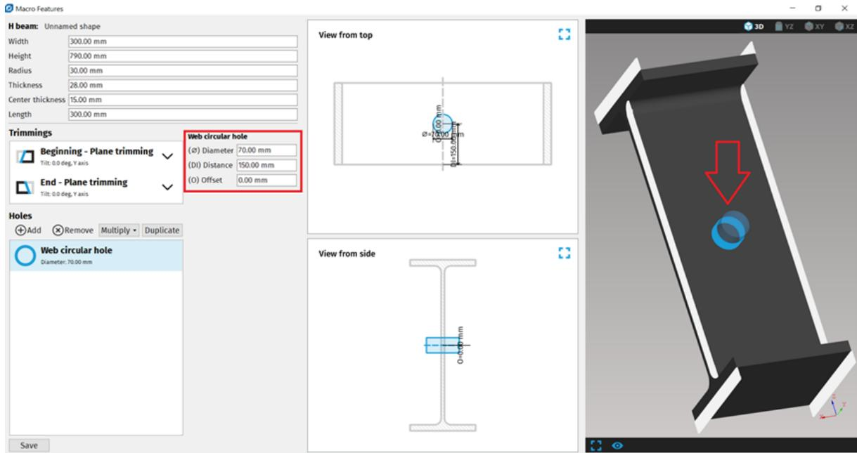
**Fig. 105: Example of Web circular hole macro placed on H beam**
