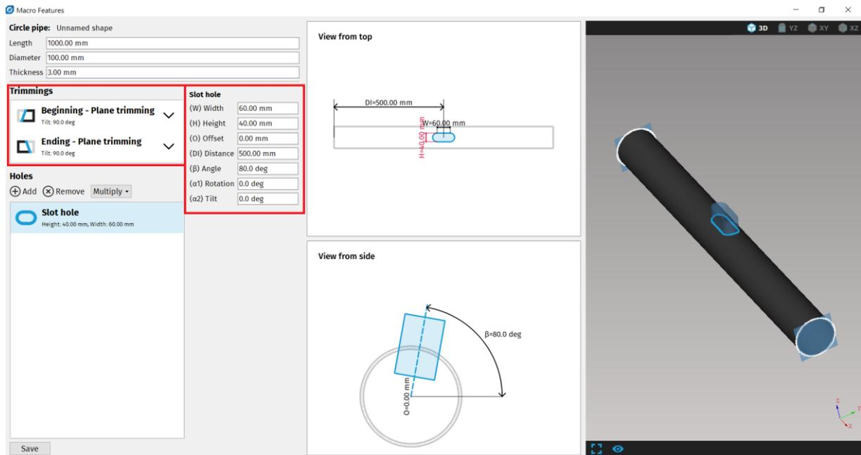
**Fig. 98: Trimmings and properties of Slot hole for circle pipe**
