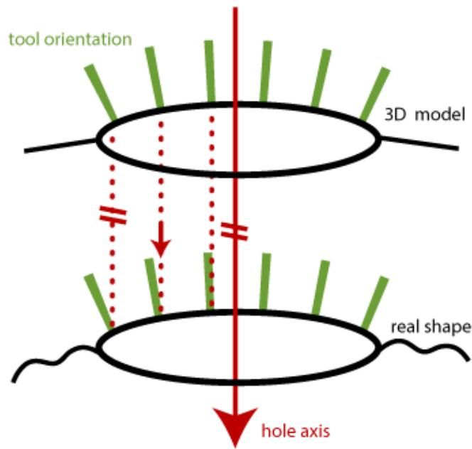
**Fig. 147: Direction of shifting the cutting path with generated hole axis**
