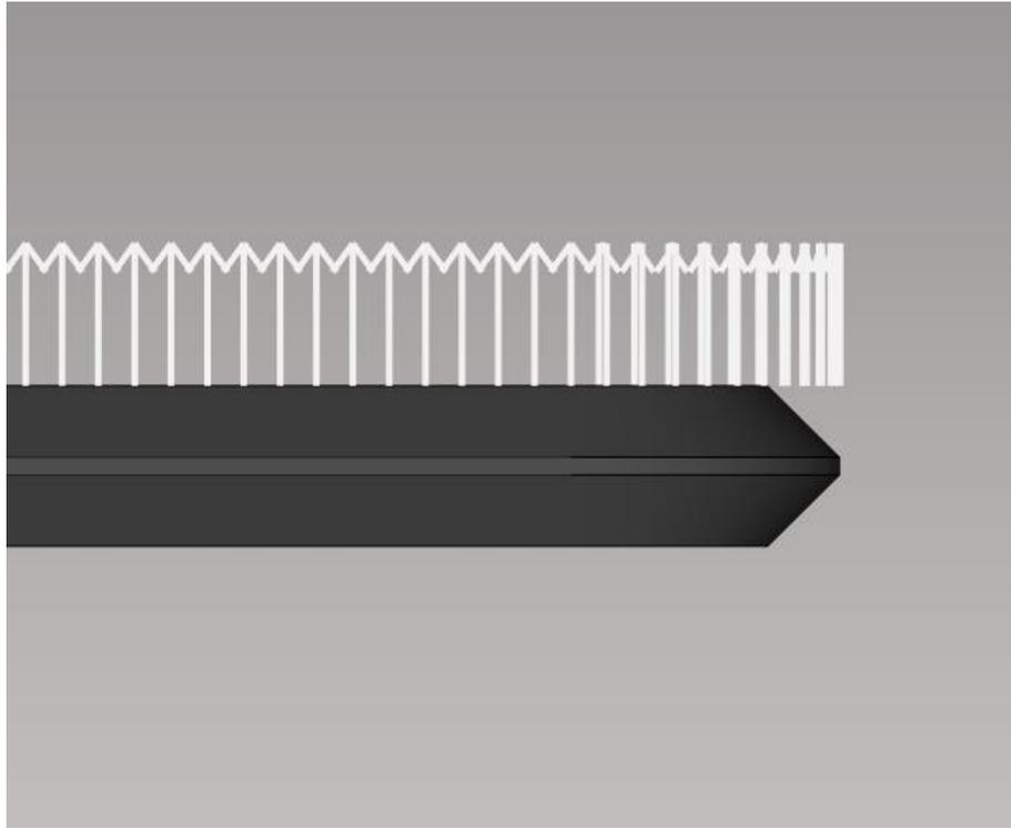
**Fig. 133: Detail of the web on tongue ending with K-cut replaced with straight cut**
