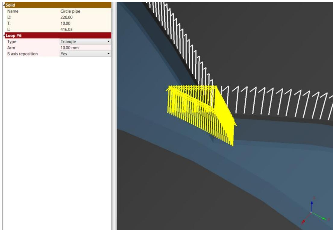
**Fig. 176: Loop type – triangle**
