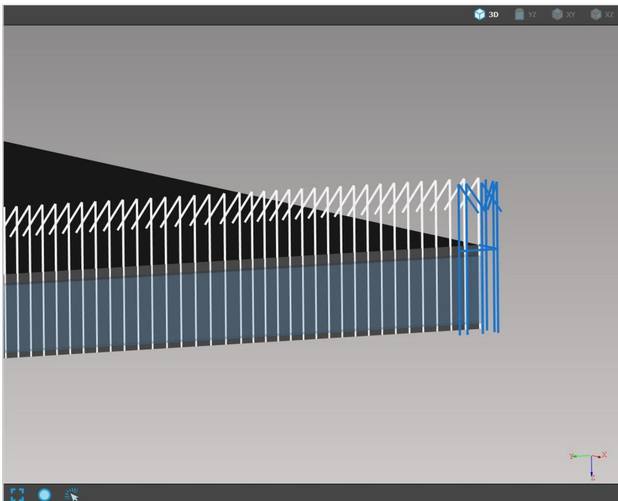
**Fig. 36: Cutting points are displayed along entire thickness of the material**
