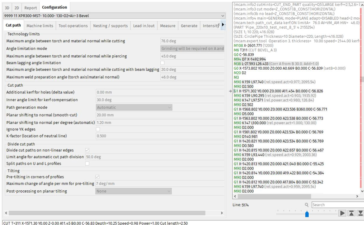
Fig. 289: Program configuration – used for CNC generation
