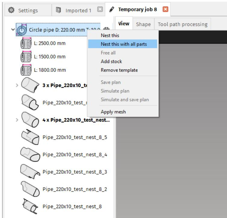
**Fig. 256: Nesting of all parts within template Circle pipe D: 220 mm, T: 10 mm**
