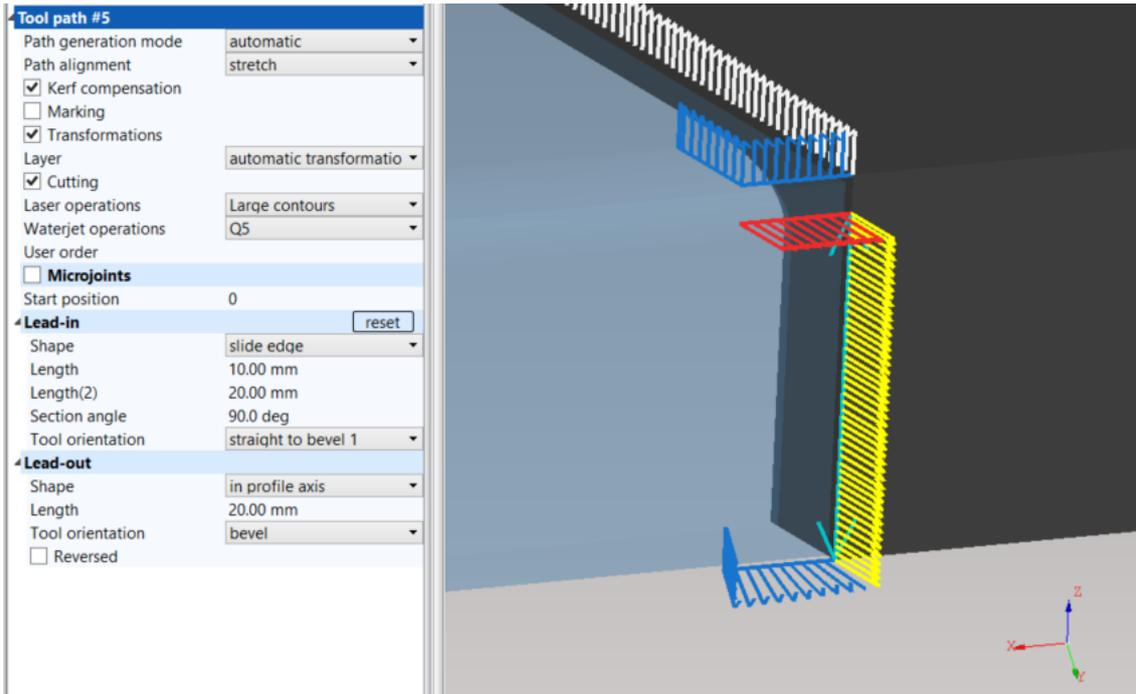
**Fig. 328: Lead-in edge slide, Lead-out in profile axis**
