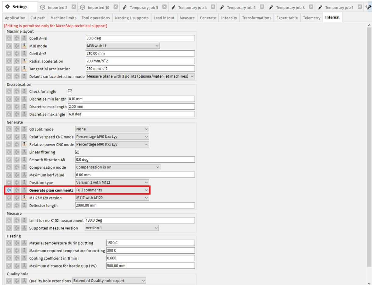
**Fig. 190: Generate plan settings in Internal section of mCAM Settings**
