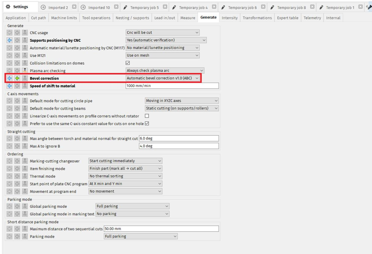
**Fig. 189: Bevel correction – Automatic bevel correction v1.0 (ABC)**
