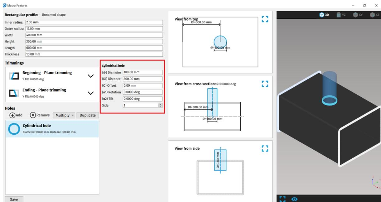
**Fig. 101: Example of cylindrical hole on rectangular profile**
