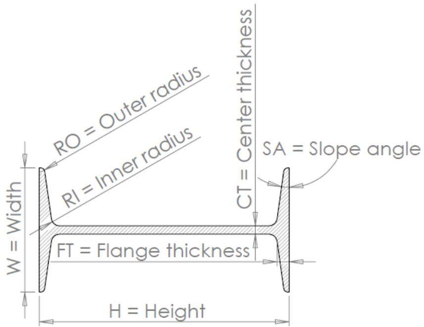
**Fig. 12: I profile - IPN beam (non – parallel flanges)**
