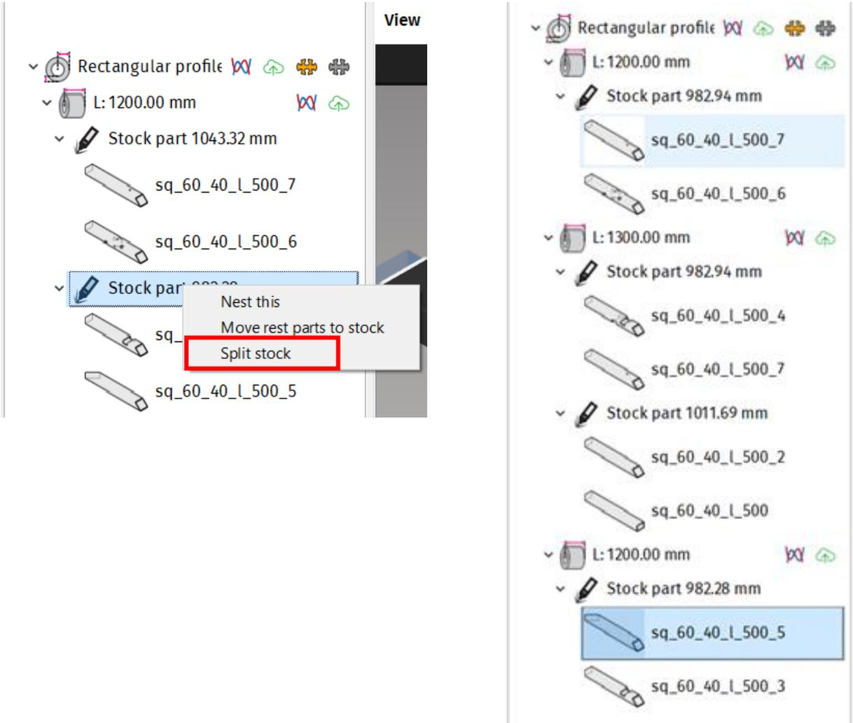
Fig. 412: Before and after “Split stock” results in mCAM
