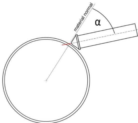
**Fig. 297: Maximum angle between torch and material normal while cutting**
