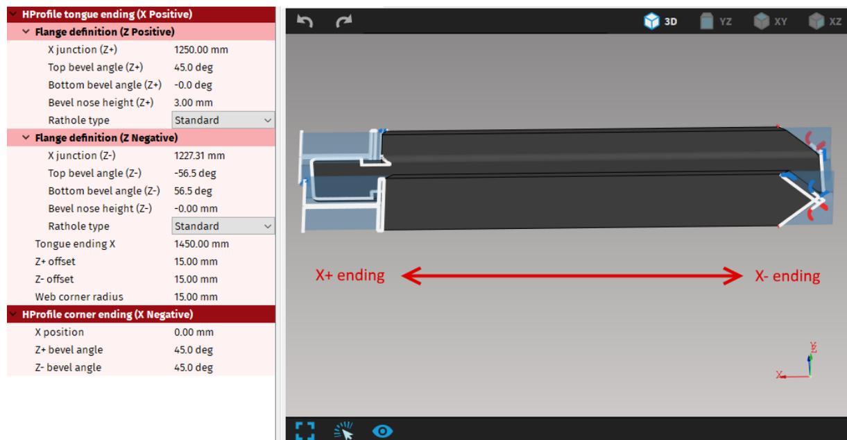
**Fig. 120:** Each part can contain maximum of two macros – One in X+ and one in X- direction
