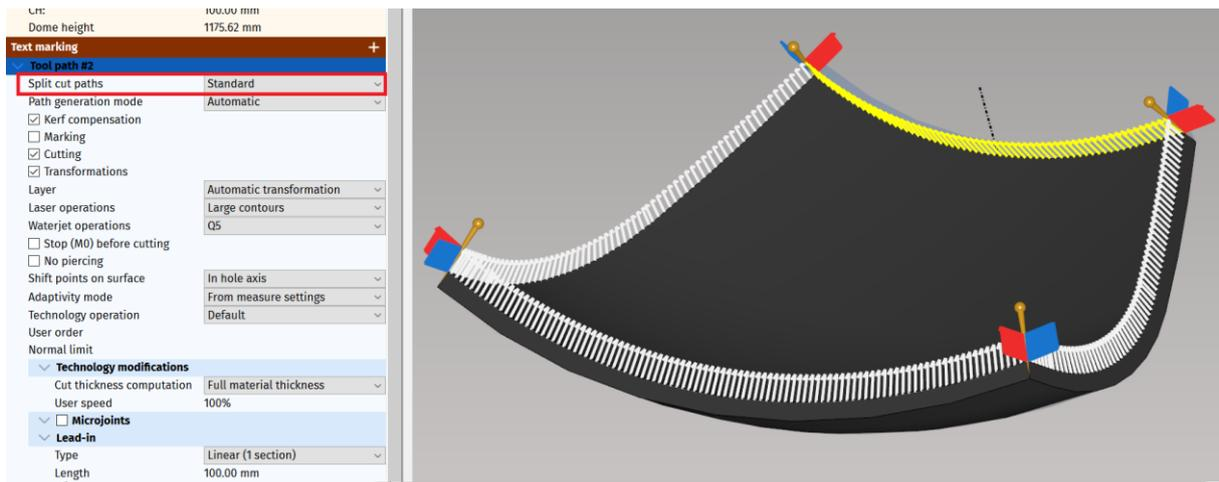
**Fig. 376: Cut paths after splitting in mCAM**
