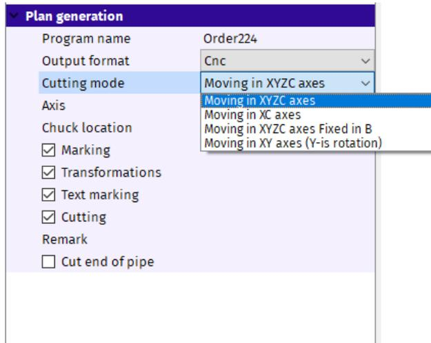
**Fig. 270: Plan generations settings – Cutting mode**
