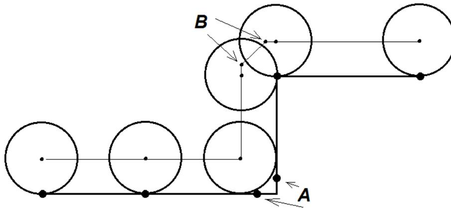
**Fig. 238: Principle of kerf width compensation**
