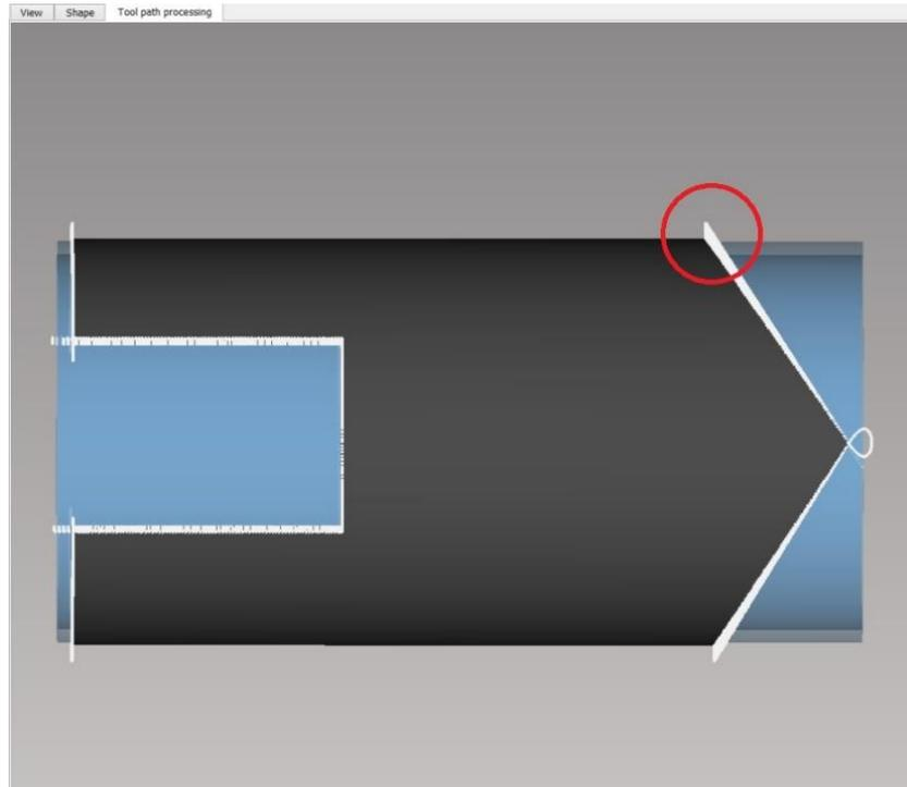
**Fig. 248: Tool path processing view (processed cutting paths) – straight cutting head limitations**
