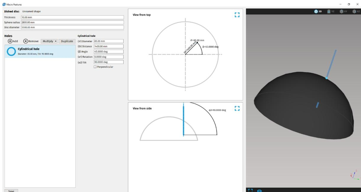
**Fig. 115: Example of cylindrical hole macro placed on dished disc dome**
