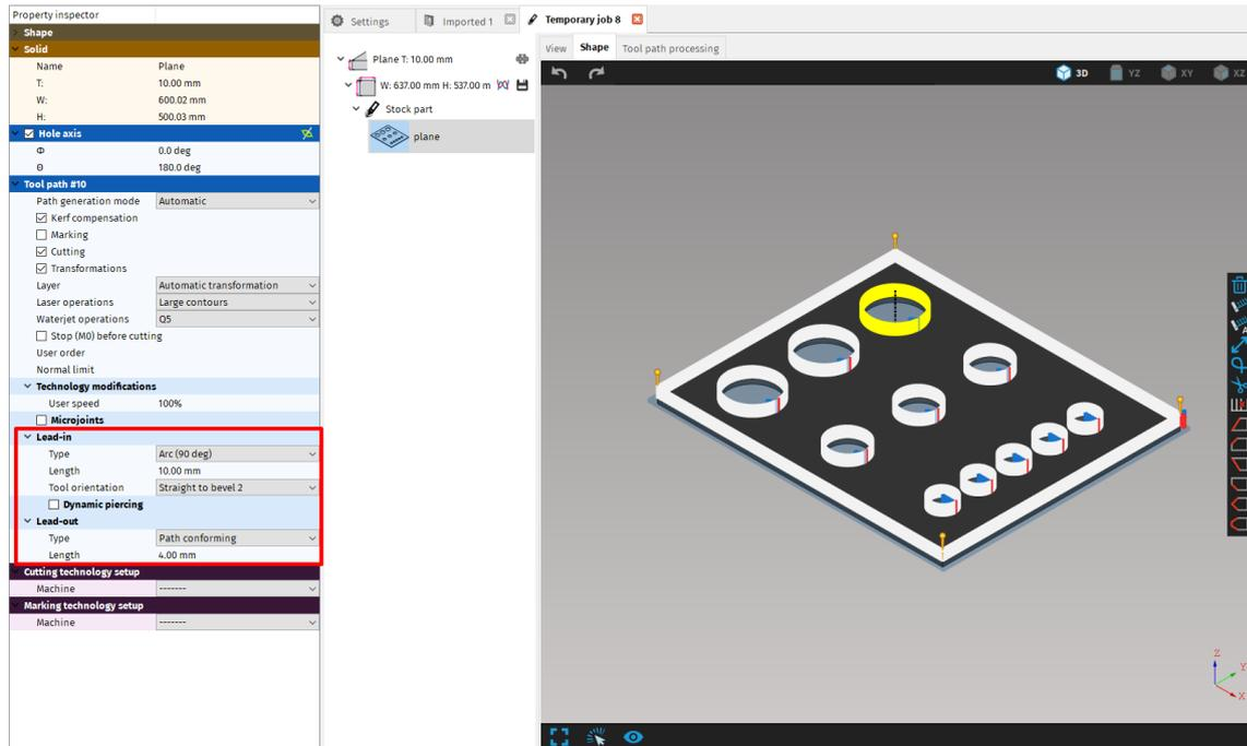
**Fig. 155: Setting the lead-in/out for selected cutting path in Properties area**
