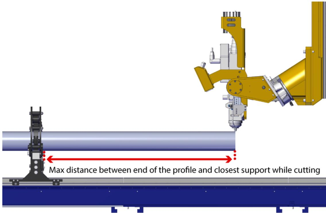
**Fig. 318: Support-End of profile distance**
