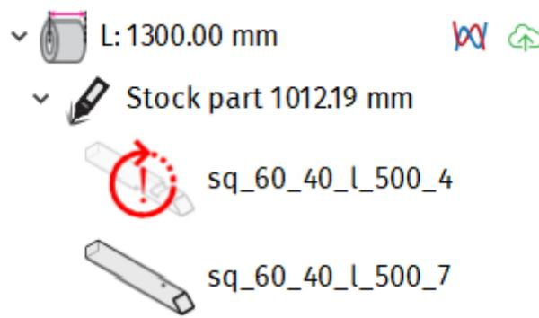
**Fig. 402: mCAM will alert the operator in case when the part can't be cut due to a limitation of the positioner**
