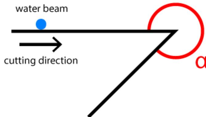
**Fig. 339: Minimum angle of contour to use relative cutting speed (WaterJet cutting)**
