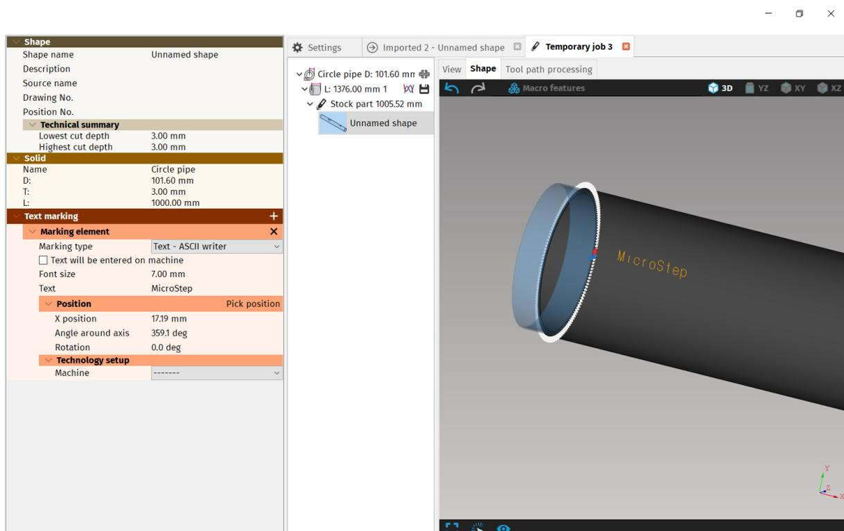
**Fig. 192: Text marking element**
