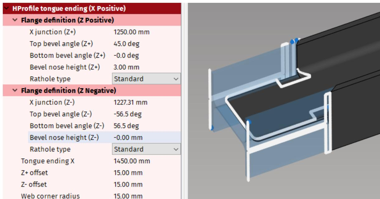
**Fig. 121: Tongue ending and its parameters in Properties area**
