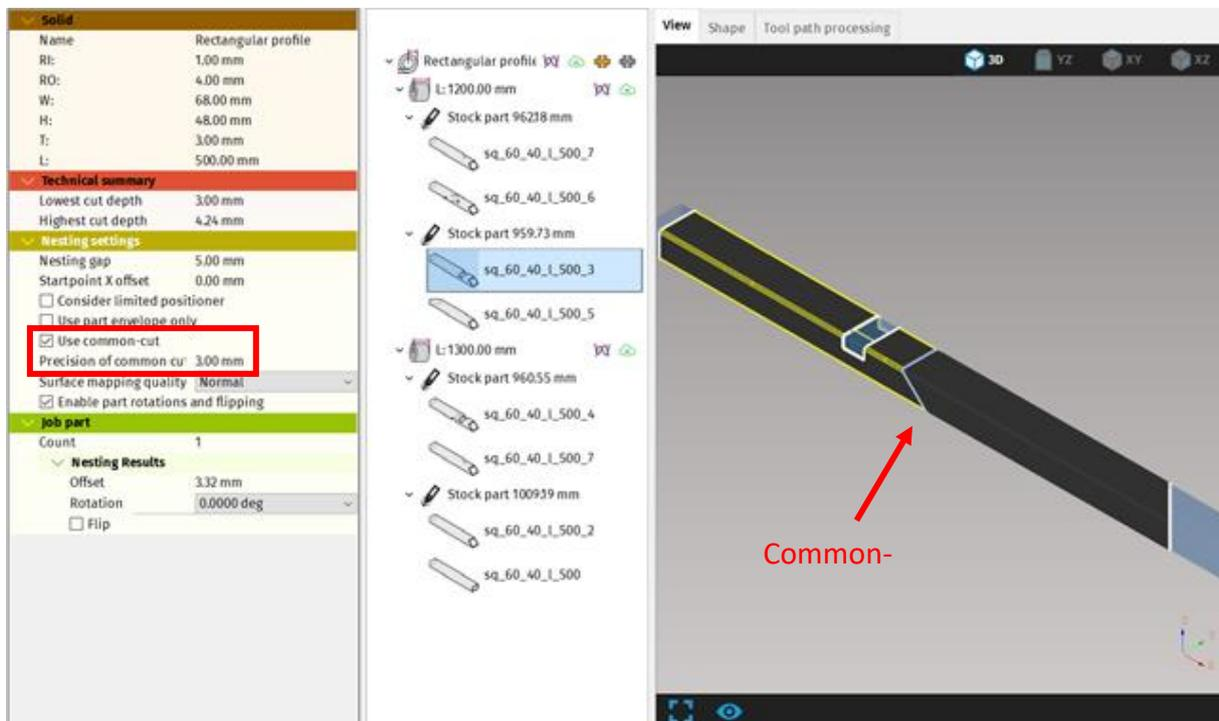
**Fig. 408: Common cut in mCAM**
