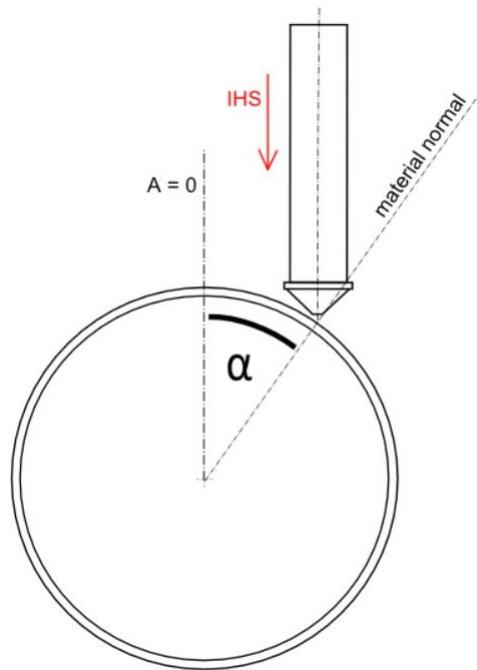
**Fig. 334: Maximum angle between material normal and up direction while surface detection**
