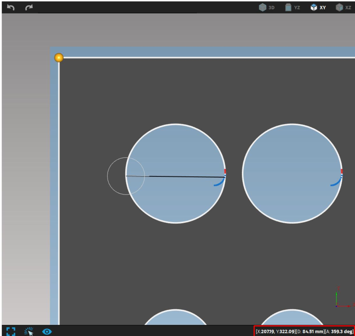
**Fig. 34: Measuring the diameter of the hole**
