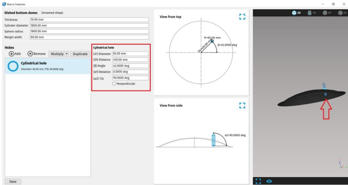
**Fig. 110: Example of Cylindrical hole macro on Dished bottom dome**
