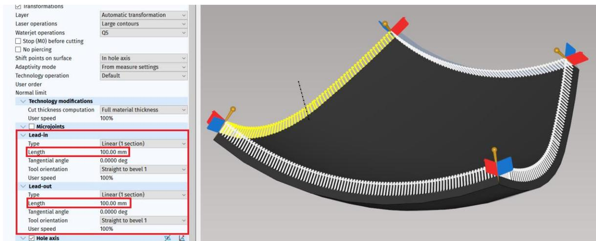
**Fig. 377: Setting the lead ins and lead outs for each cutting path in mCAM**
