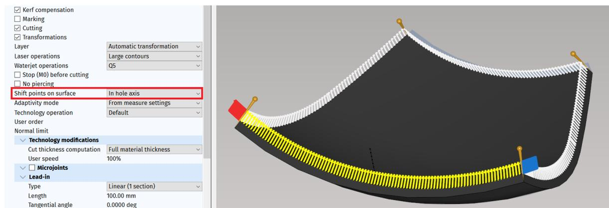
**Fig. 385: Shift points on surface – in hole axis type in mCAM**
