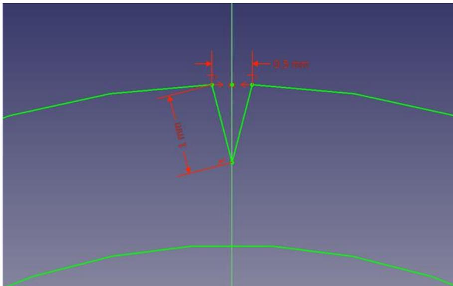
**Fig. 211: Groove profile on the outer surface of circle pipe**
