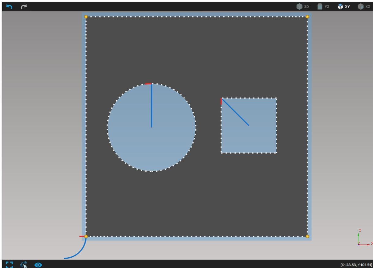
**Fig. 320: Lead-ins on small holes begin in the center of the hole**
