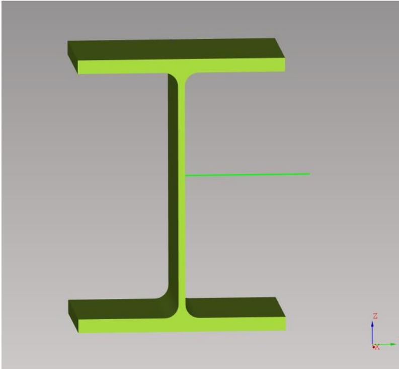
**Fig. 74: H-bar – (older position) top edge of cutting contour, where the cutting starts, needs to be in Y+ direction, the flanges are in Y-axis**
