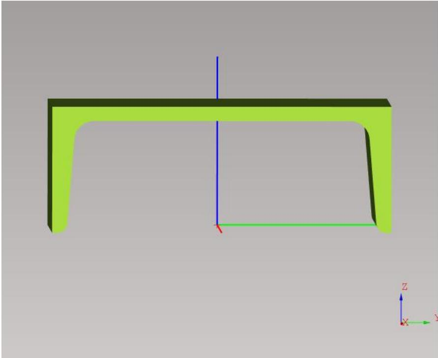
**Fig. 79: UPN-bar – Flanges are in Z-axis, with web facing Z+ direction (new position)**
