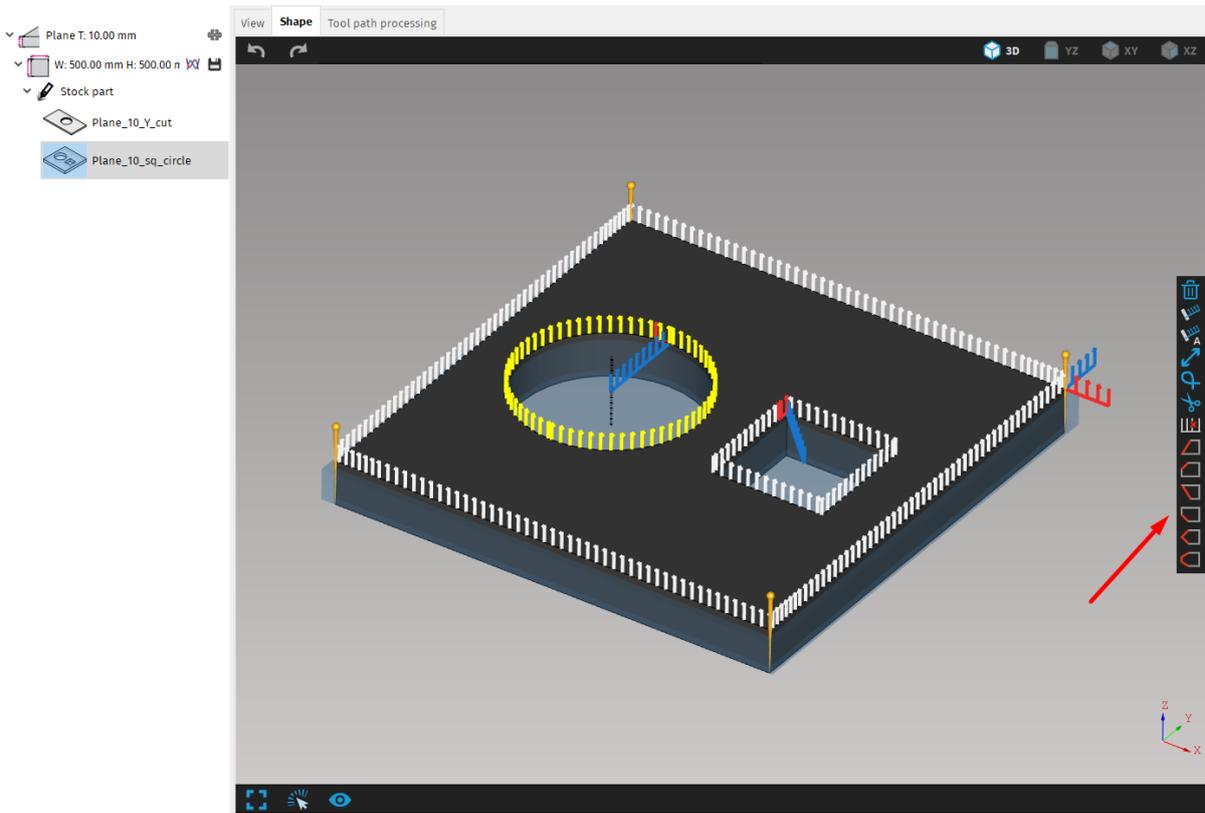
**Fig. 202: Panel with various options including welding preparations shows up on the right side of the screen when the cut path is selected**
