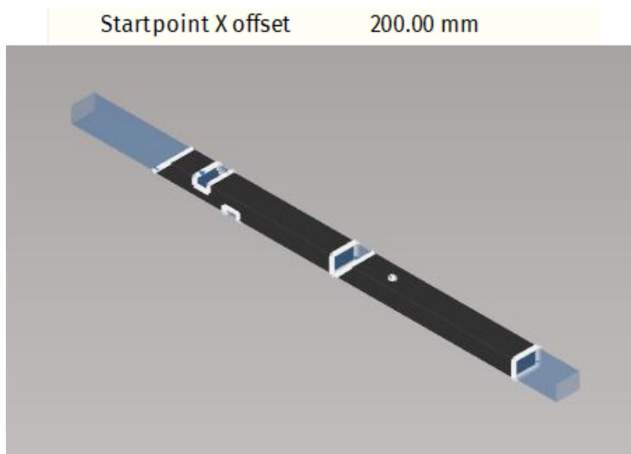
**Fig. 405: Start point X offset option applied on the material**
