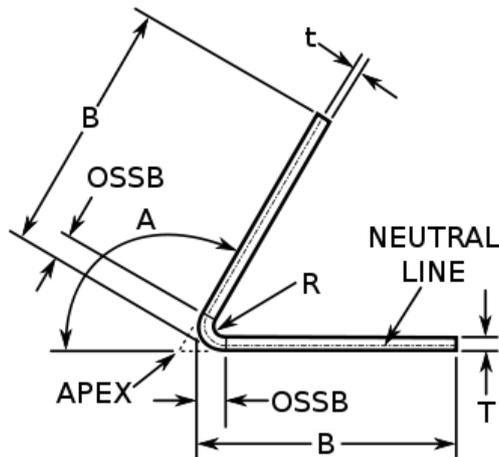
**Fig. 303: Definition of K-factor for bending (<http://www.wikipedia.org>)**
