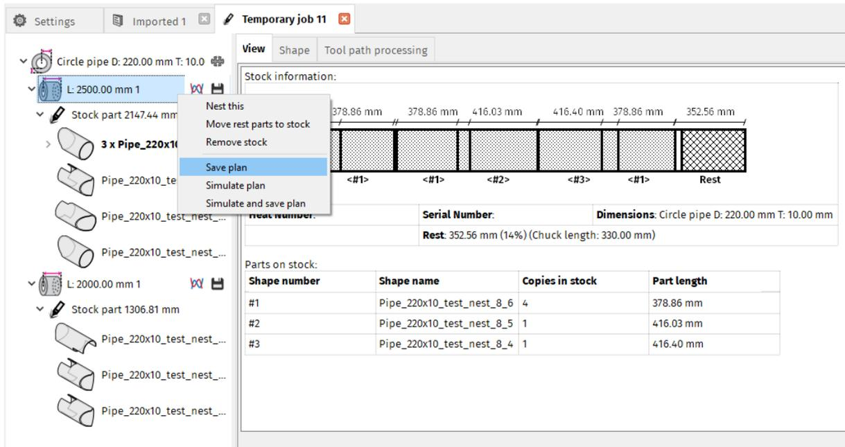
**Fig. 277: Save cutting plans for stock with length 2500 mm**
