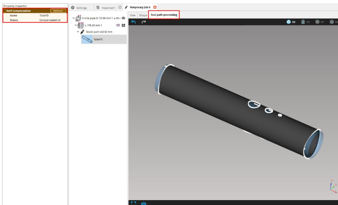
**Fig. 245: Tool path processing (compensated and limited paths)**
