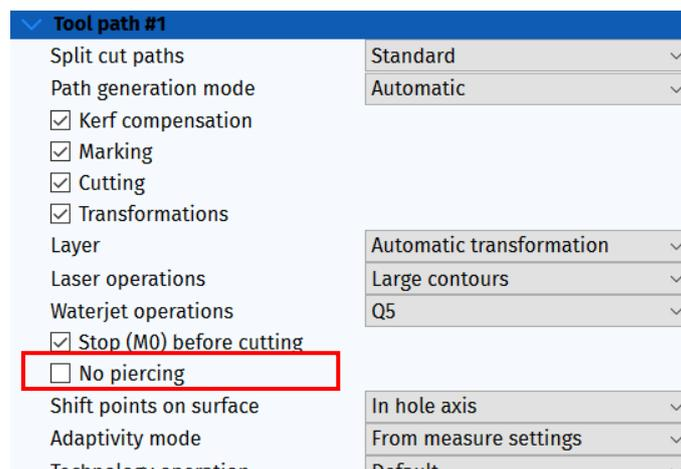
**Fig. 381: Stop before cutting the checkbox in mCAM**
