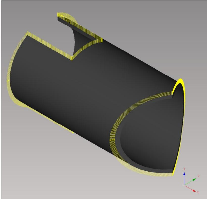
**Fig. 246: Raw-processed cutting paths (according to input settings and applied path-generation mode)**
