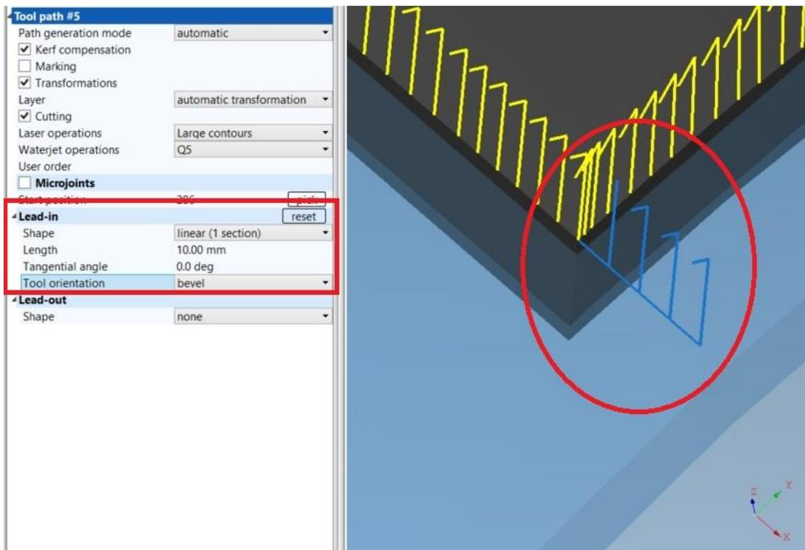
**Fig. 330: Tool orientation – bevel**
