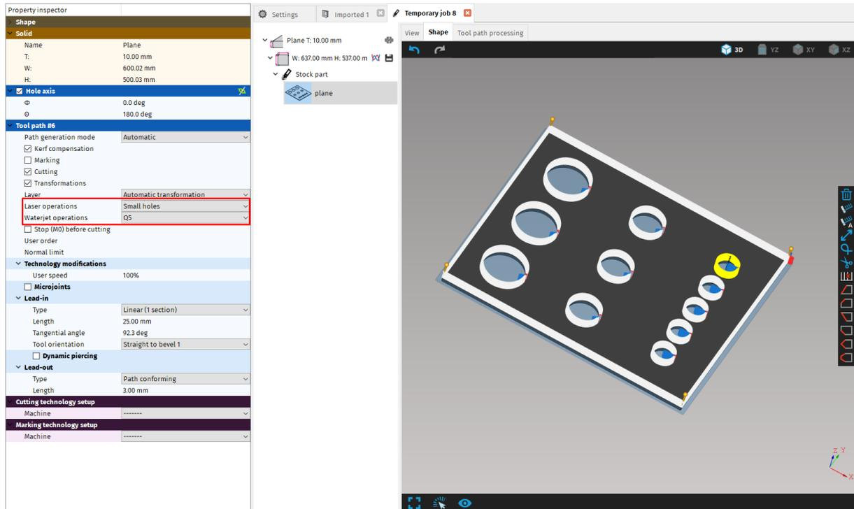
**Fig. 199: Tool operation settings (for laser or water jet cutting)**
