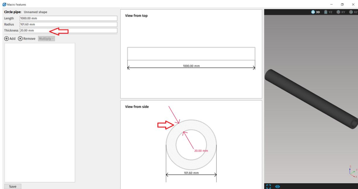
**Fig. 93: How to change shape's dimensions**
