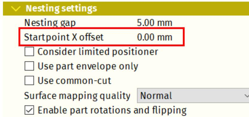
**Fig. 404: Start point X offset option in mCAM**
