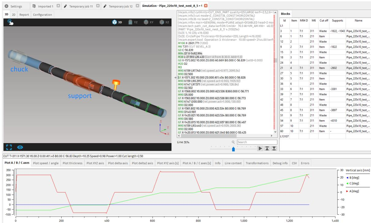
**Fig. 280: 3D simulation with highlighted chuck location and support position**
