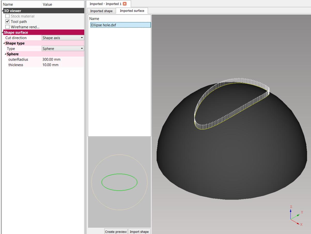
**Fig. 47: Importing of projected 2D surface on sphere–cap**
