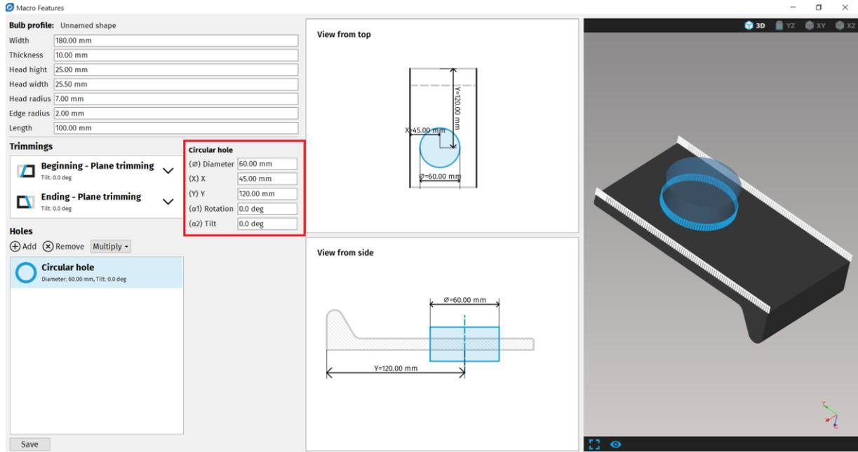
**Fig. 102: Properties of Circular hole for Bulb profile**
