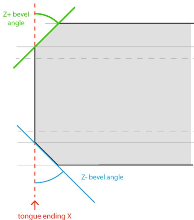
**Fig. 131: Top view of corner ending welding connection with its parameters**
