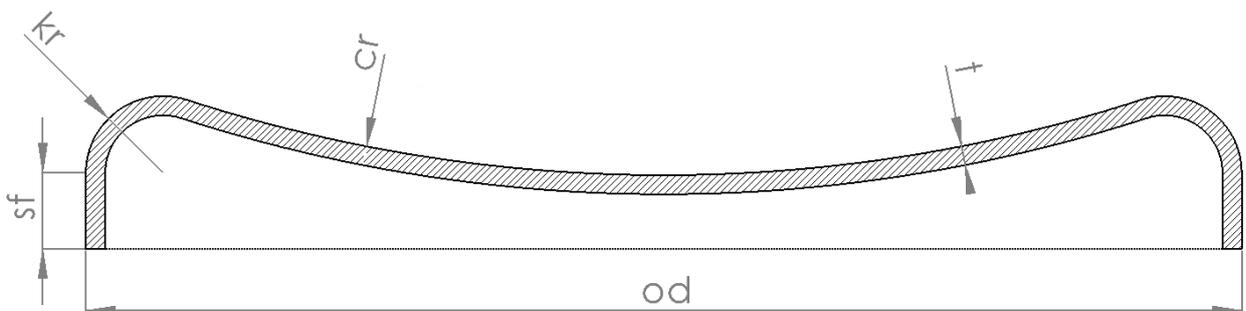
**Fig. 24 Inverted head dome**
