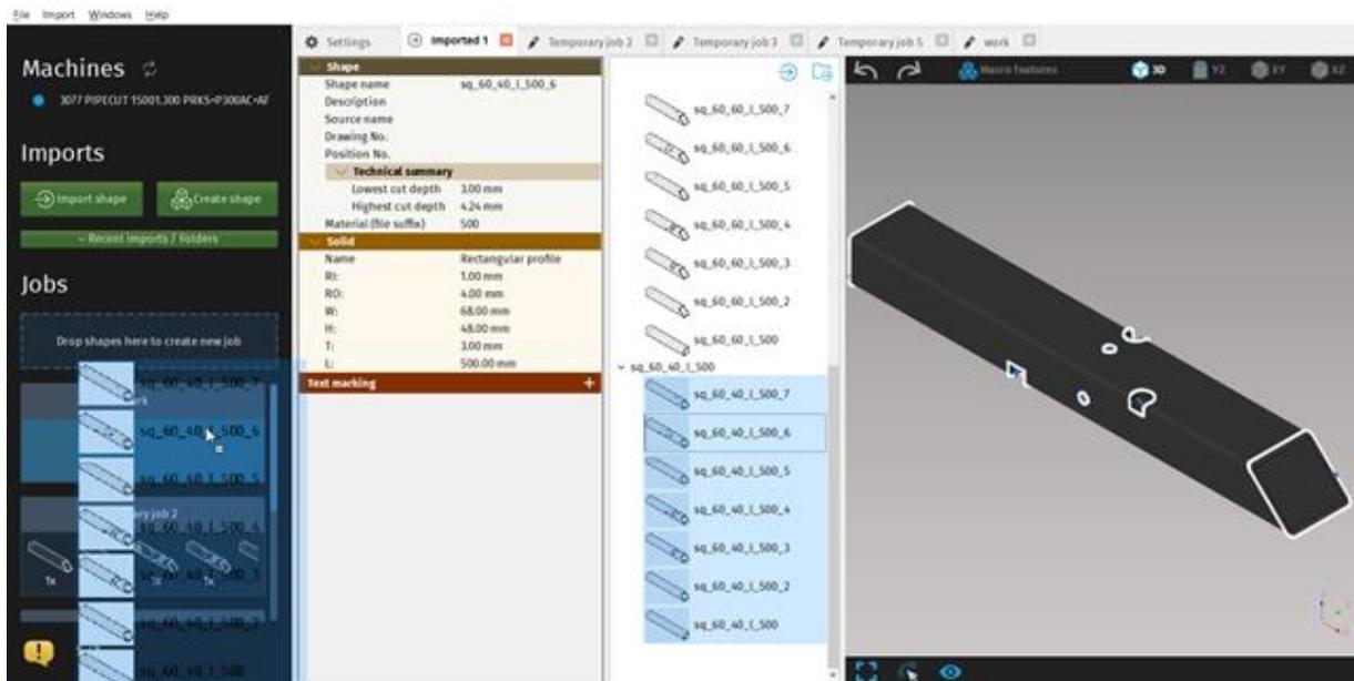
**Fig. 392: Drag shapes into already created Job in mCAM**
