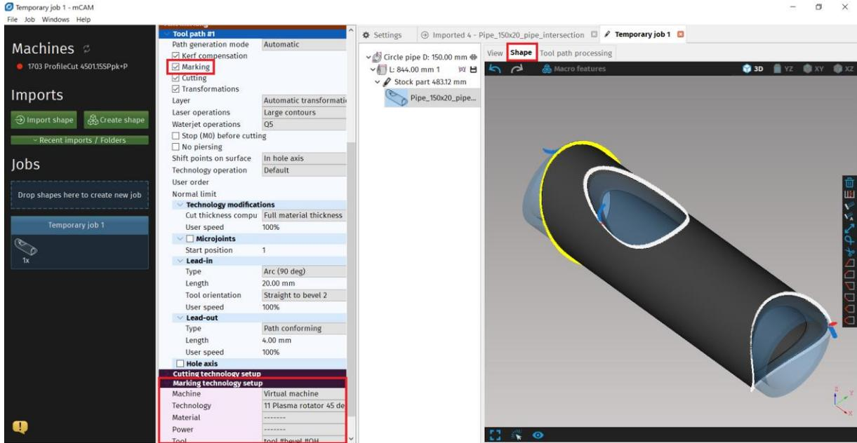
**Fig. 186: Marking is enabled for selected cut path and plasma technology with respective tool is selected in Properties area**
