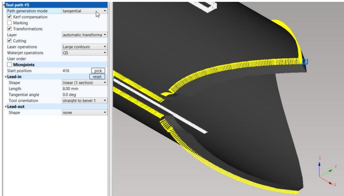
**Fig. 162: Tangential tracking of cutting path – tangential mode**
