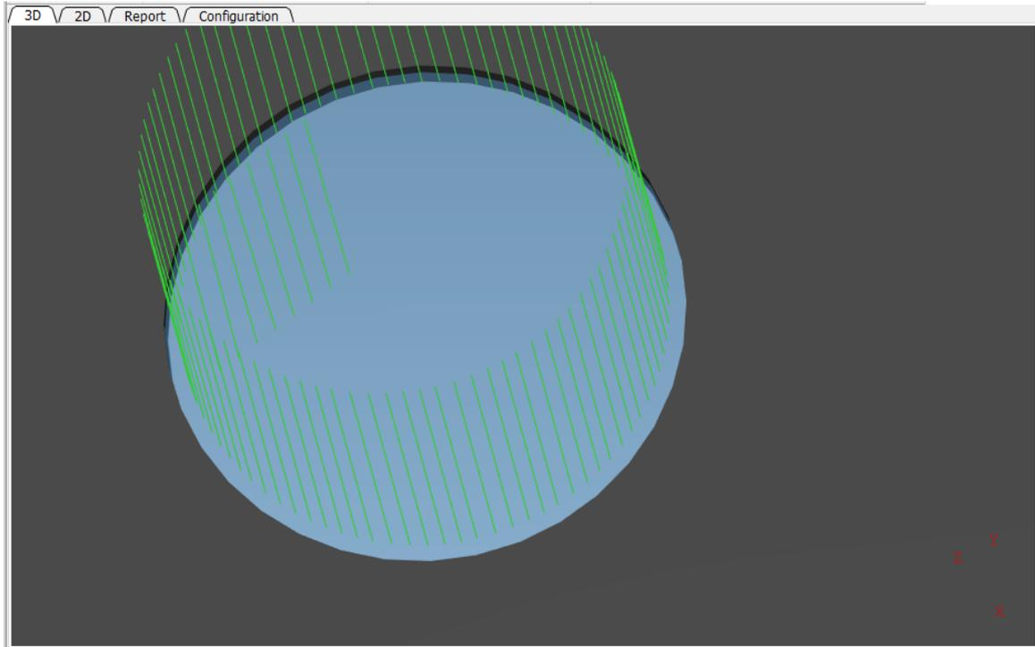
**Fig. 171: Kerf width compensation on the inside of the hole while the cut path is not reversed.**
