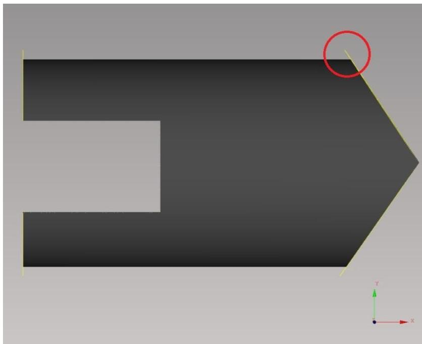
**Fig. 247: Side-view on raw-processed cutting paths (bevel cutting)**
