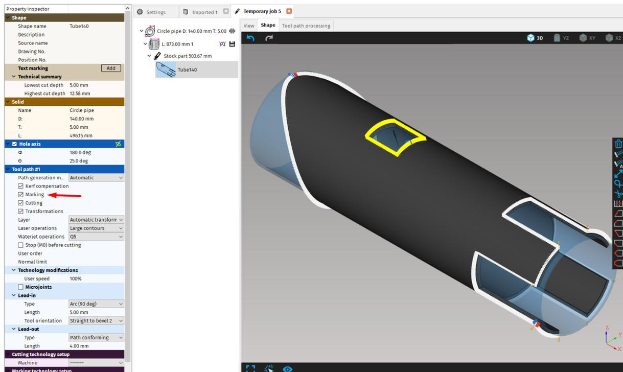
**Fig. 157: Marking of cutting contour**
