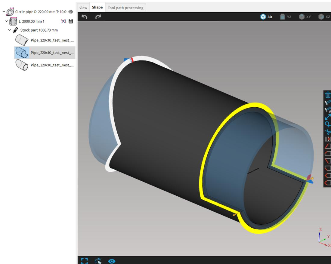
**Fig. 32: Cutting path selection in visualization screen**
