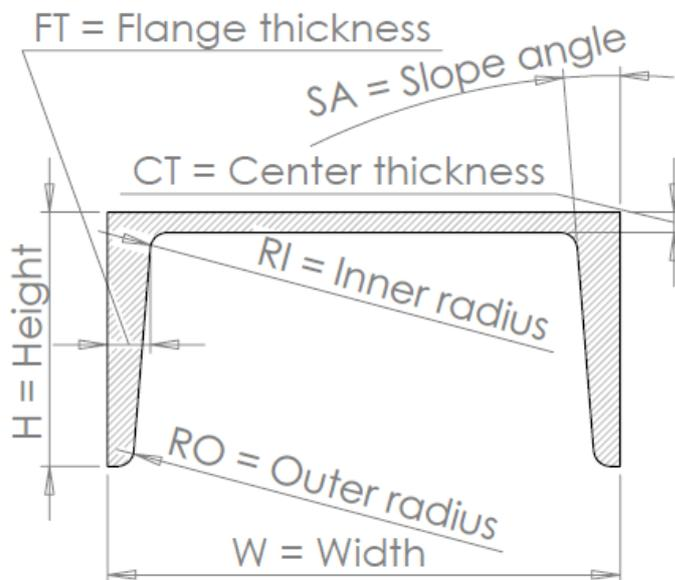
**Fig. 15: UPN beams (non – parallel flanges)**
