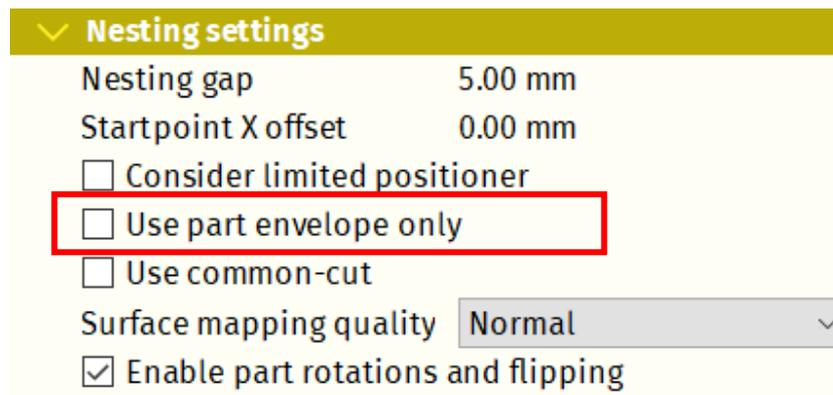
**Fig. 406: Option “Use part envelope only” in mCAM**
