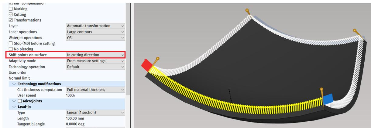
**Fig. 387: Shift points on surface – in cutting direction type in mCAM**
