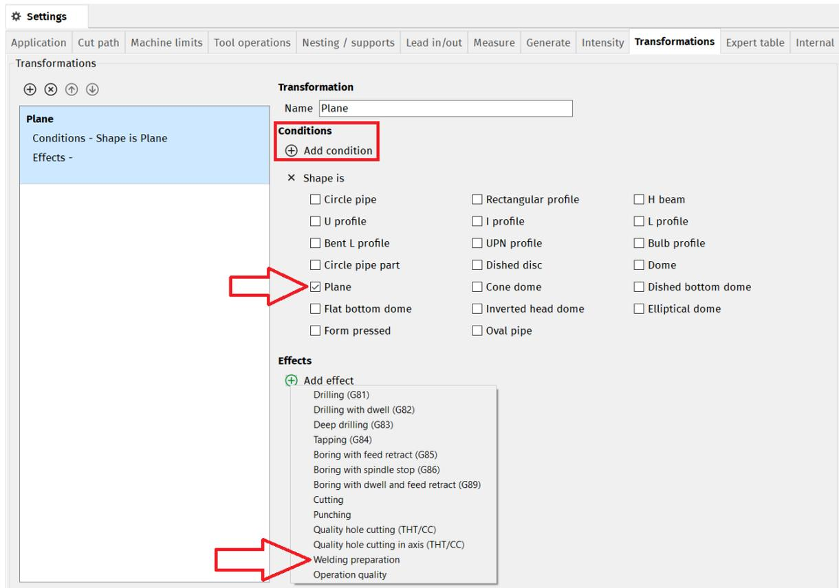
**Fig. 206: Welding preparation in Transformations section of mCAM Settings**
