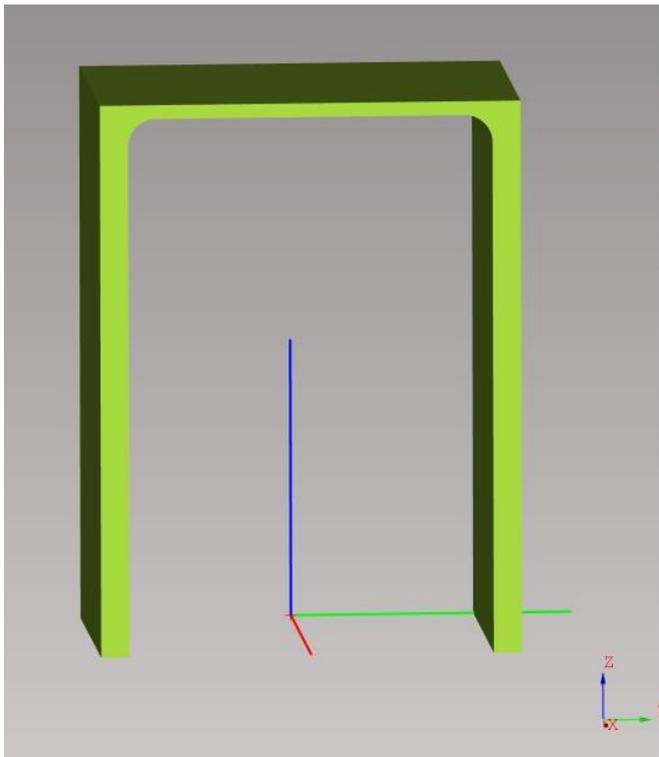
**Fig. 77: U-bar – Flanges are in Z-axis, with web facing Z+ direction (new position)**
