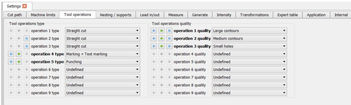
**Fig. 197: Standard laser tool operations setup**
