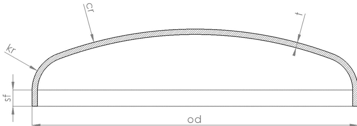
**Fig. 19: Torospherical dome**
