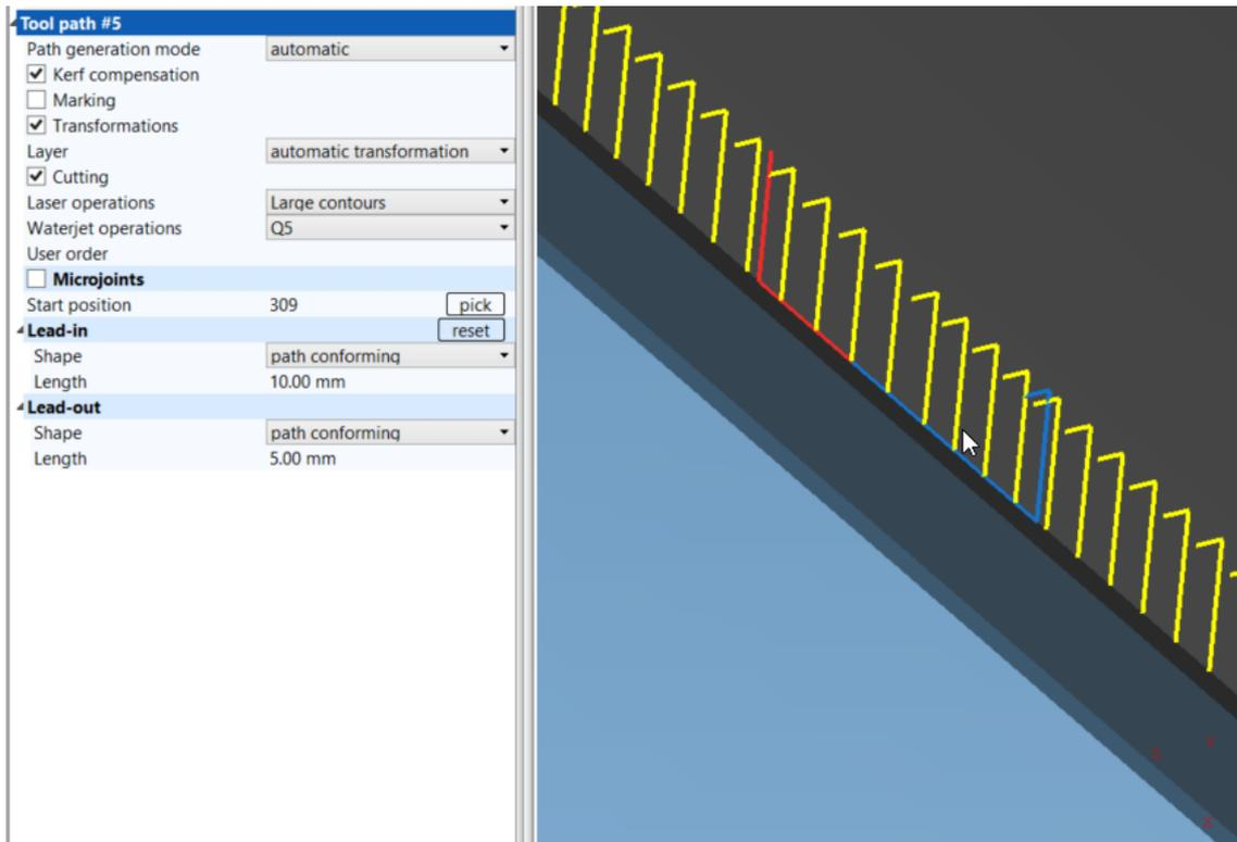
**Fig. 322: Lead-in path conforming, lead-out path conforming**
