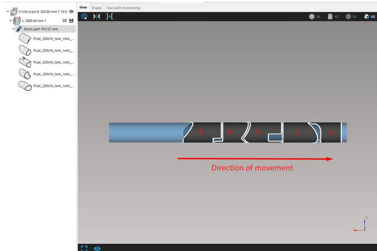
**Fig. 265: Direction of movement of parts in active manual nesting mode in XZ view**
