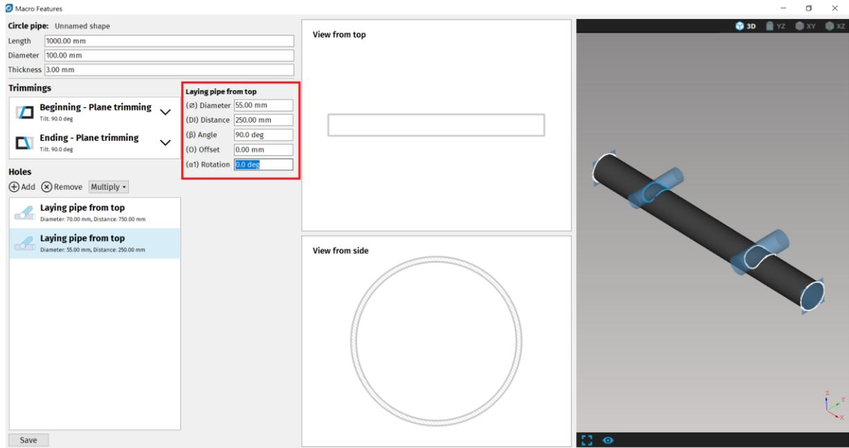
**Fig. 99: Properties for Laying pipe from top in Macro features**
