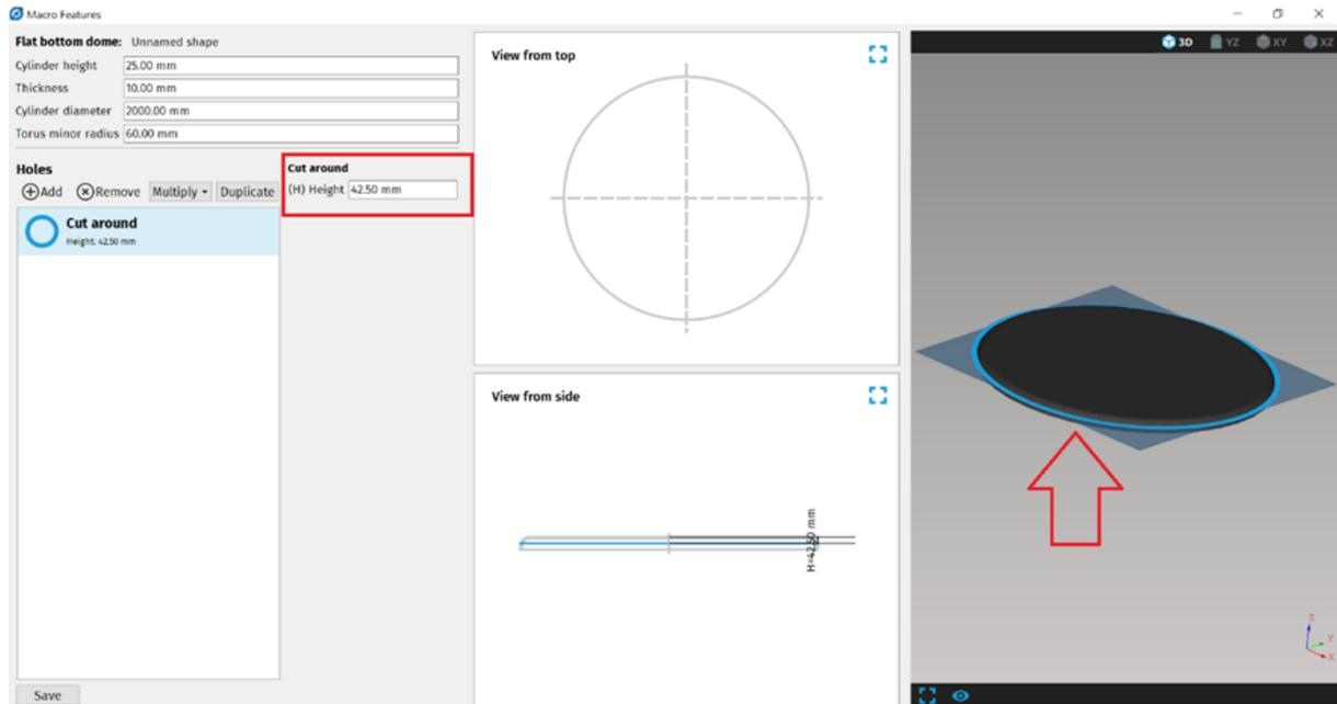
**Fig. 109: Example of Cut around macro placed on Flat bottom dome**
