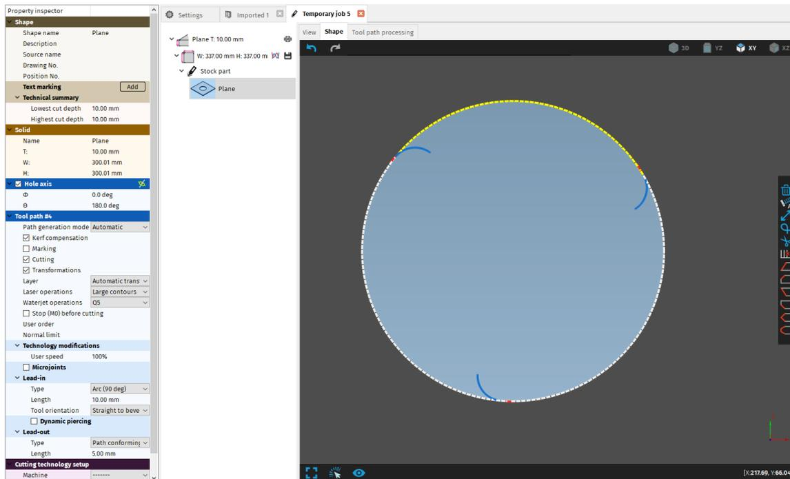
**Fig. 237: Cut path split to three parts**
